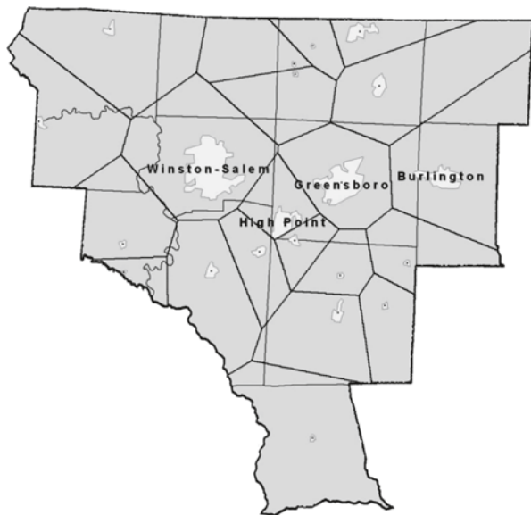
Fig. 19.12 Unweighted Voronoi diagram with \ell_2 distances
