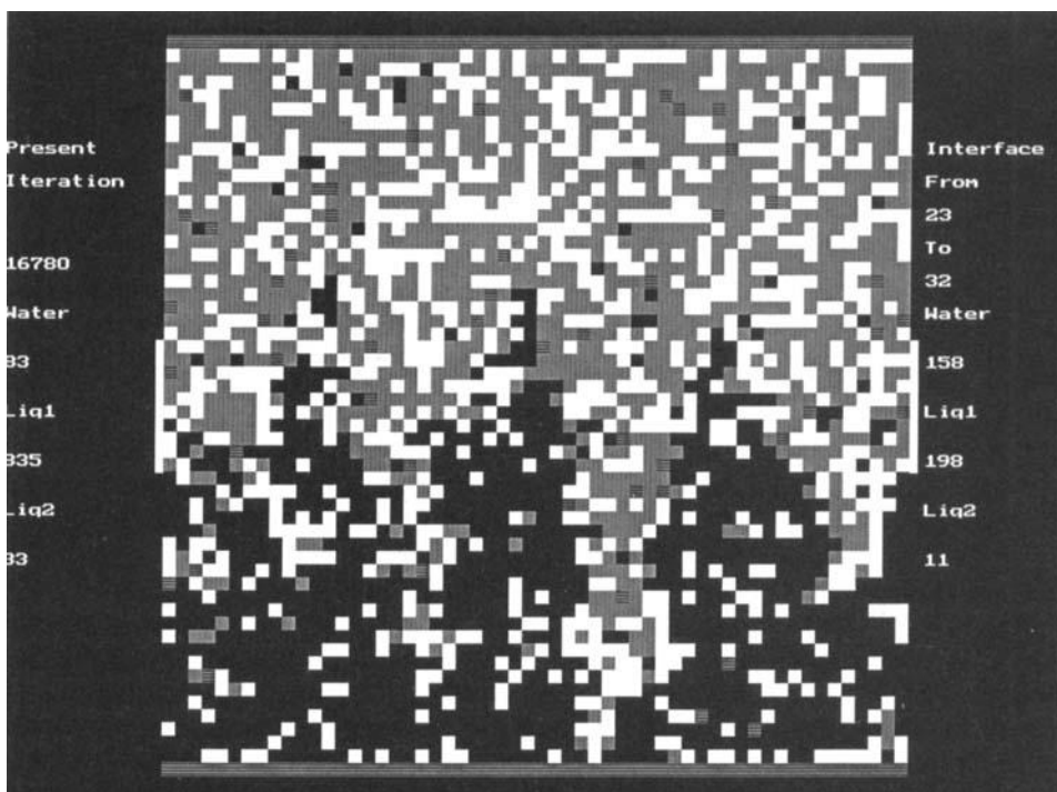
Figure 6. A well-developed model of the immiscible liquid interface showing the preference of the solute for the nonpolar liquid. Note the extensions of each liquid in the other phase
