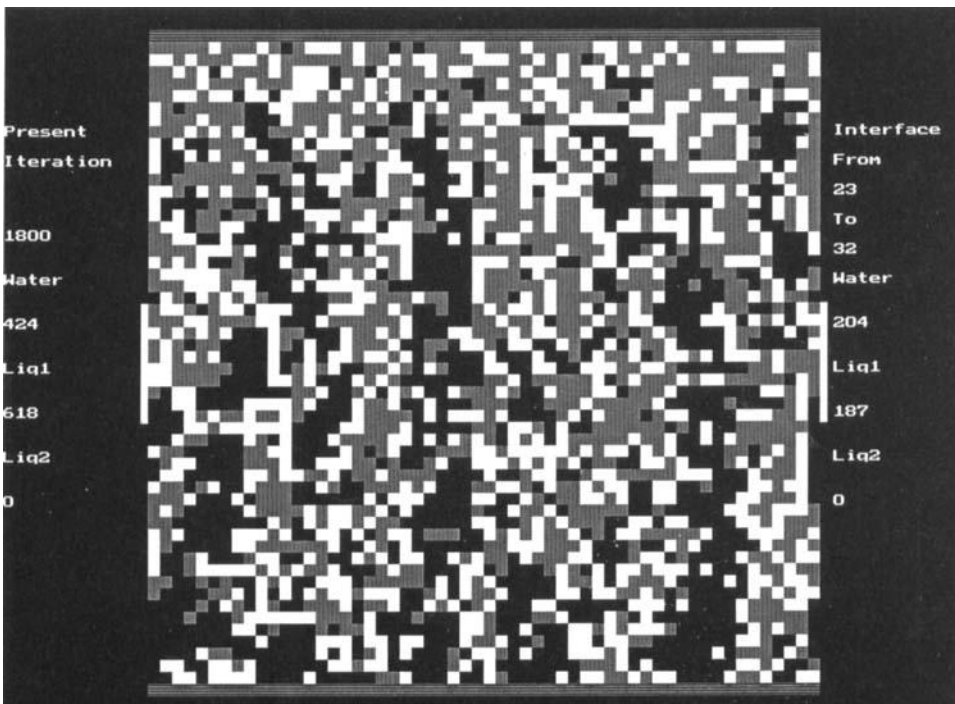
Figure 2. The partial separation of two immiscible liquids showing the elongated stacks of each liquid. The water is black, the nonpolar liquid is gray and the cavities are white
