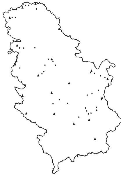
Figure 4. Distribution of undulation determined by the GPS/dh method (triangles for fitting, black marks for external checking).
