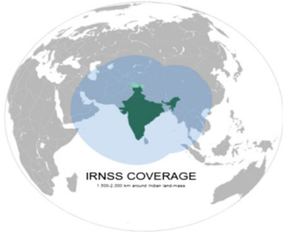
Fig. 1 IRNSS coverage area about 1500 km around the Indian land mass (image credit from ISRO)
