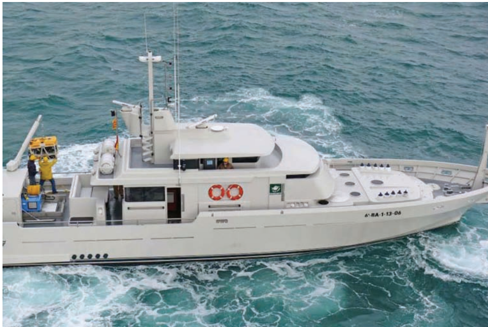
Fig. 12.23 Modern survey vessel specially adapted for ROV inspection to 400 m of water depth, belonging to Argo Maris Private Foundation. Propulsion is by hull-mounted jets instead of propellers, which ensures safer operation at sea. Note the ROV hangar (in open position) to the left and small crane above it. The boat needs only three crew. This vessel is often used by GRC Geociències Marines from the University of Barcelona, which also uses other specially adapted vessels for high-resolution mapping, inspection and sampling of the continental shelf floor. Argo Maris Private Foundation.
