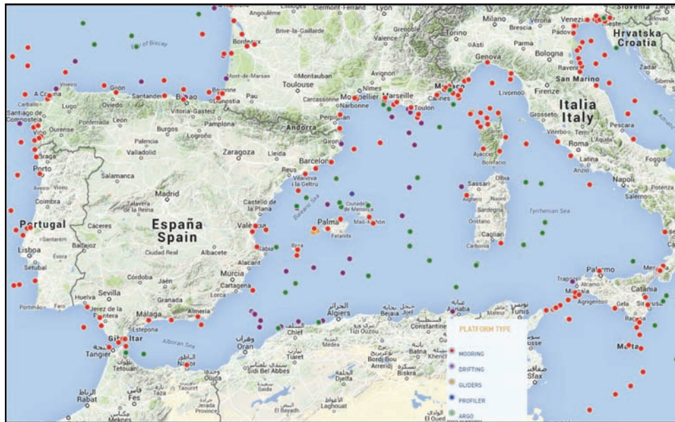
Fig. 12.16 Screenshot of EMODnet showing the distribution of moorings (including metocean buoys), drifting buoys, gliders, profilers and Argo floats in the western Mediterranean Sea since 1950. An on-line query option in the EMODnet website allows access in real time to the meta data of every component of the observational network, including types of data lists. Time-series data from the different private and public organizations is also available to download from the EMODnet website ( www.emodnet.eu/ ).
