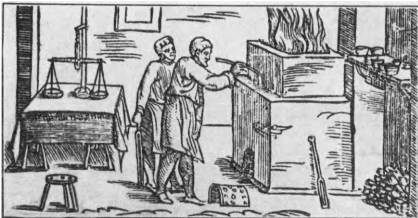
FIG. 4. Gold testing in the 15th century. (From Biringuccio: Pirotechnia [1540])
