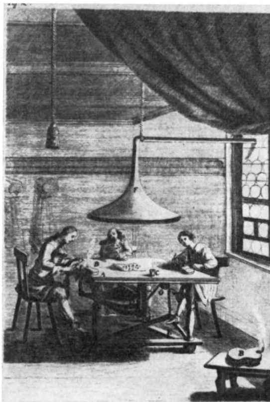
FIG. 14. Glass blowing works in the 17th century. The person on the left works with a blow-pipe. (From Kunckel: Ars vitraria experimentalis oder vollkommene Glasmacherkunst [1679])
