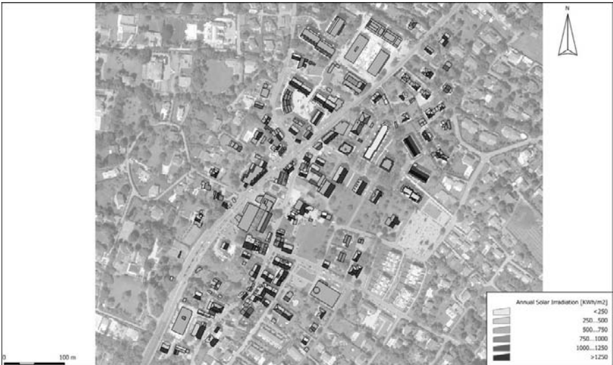
Fig. 18. Annual solar irradiance values (KWh/ m 2 ) for the second pilot zone
