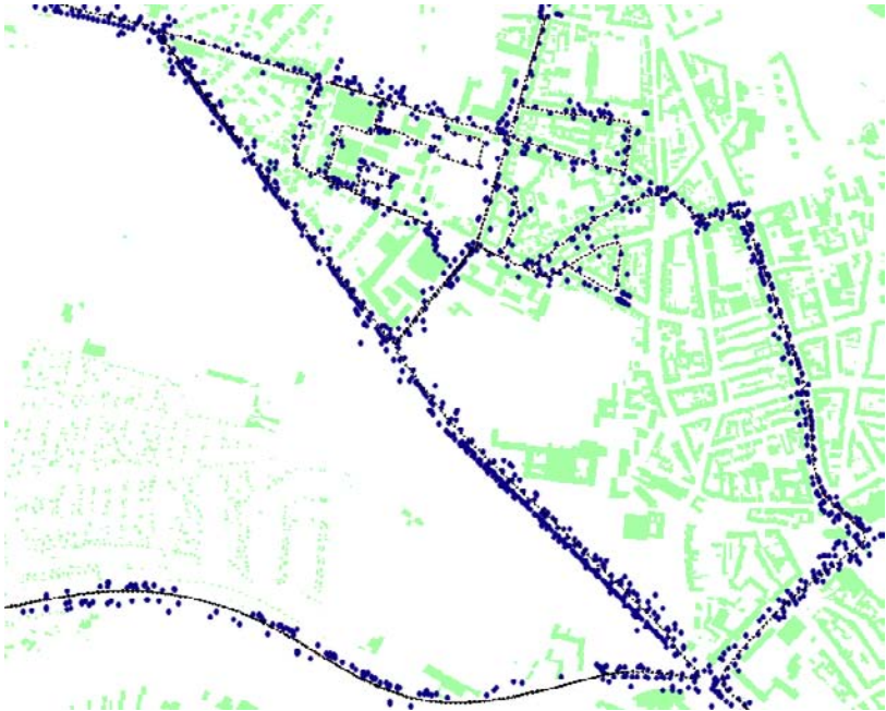
Fig. 6. Extracted poles (blue dots) in a larger area with buildings from the cadastral map (green). The thin dotted line is the trajectory of the Streetmapper van.
