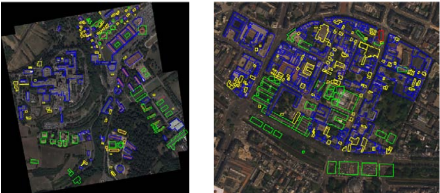
Fig. 15. Evaluation in Toulouse (left) and Amiens (right). TP cases are depicted in green, FN cases in red, FP in yellow and TN in blue.
