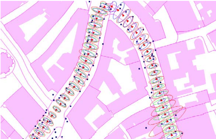
Fig. 11. Same scene as Fig. 10, for a scanner opening angle of 100° and a scan range of 50 m (red), 100 m (green), and 150 m (blue).
