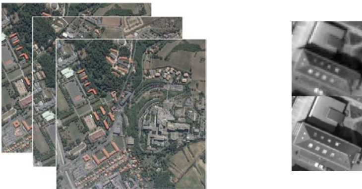
Fig. 2. Left: a triplet of Pléiades-HR images (simulations). Right: Zoom in. Pléiades-HR Simulations (top) are computed from 25cm airborne images (bottom).
