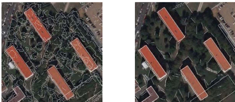
Fig. 5. 2D contours (in white, left) and 3D primitives (in white, right) are superimposed on the RGB orthophoto. Contrary to 2D contours, the extraction of 3D segments is reliable, even in challenging vegetated areas.
