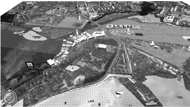
Fig. 6. Screenshot of the prototypic 3D Land Information System with integrated geodata including nature protection areas as raster-based terrain texture, water protection areas and polluted land cadastre as vector-based terrain textures.
