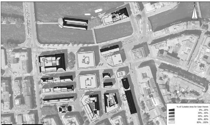
Fig. 15. Percentage of suitable area for solar panels on the first pilot zone with a Sky View Factor (SVF) of 60%
