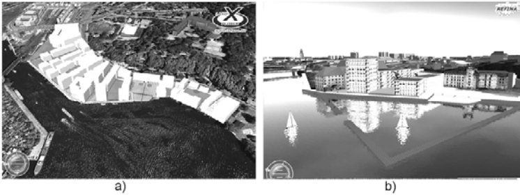
Fig. 7. The left image shows the result from using extrusion functions to create interactive block buildings and the right image shows a plan representation derived from the 3D modelling approach combined with a water shader.
