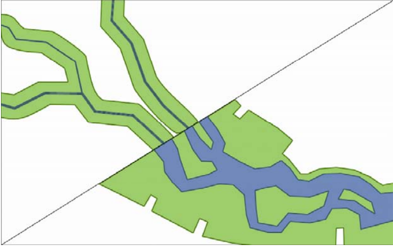
Fig. 1. A direct comparison of two geographical datasets with different geometric attributes for the same Feature Type ( River ) and different classification rules applied ( Floodplain )
