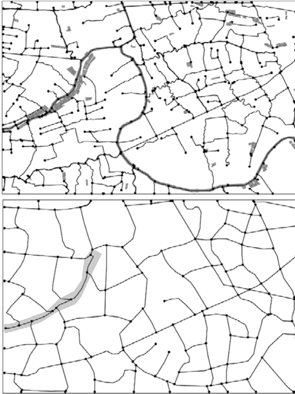
Fig. 10. The original datasets (grey) overlaid by the result of the construction of the topological correct line networks (black): (top) large-scale dataset DLG 50 and (bottom) small-scale dataset DLG 250.
