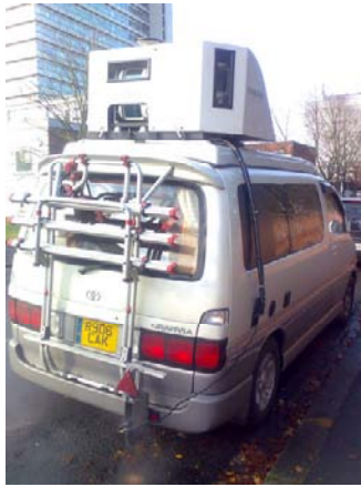
Fig. 1. The Streetmapper system used to acquire the Hannover scan. Three of the four scanners, the GPS antenna, and the odometer (mounted close to the bumper) can be discerned. The fourth scanner pointing to the left is occluded.
