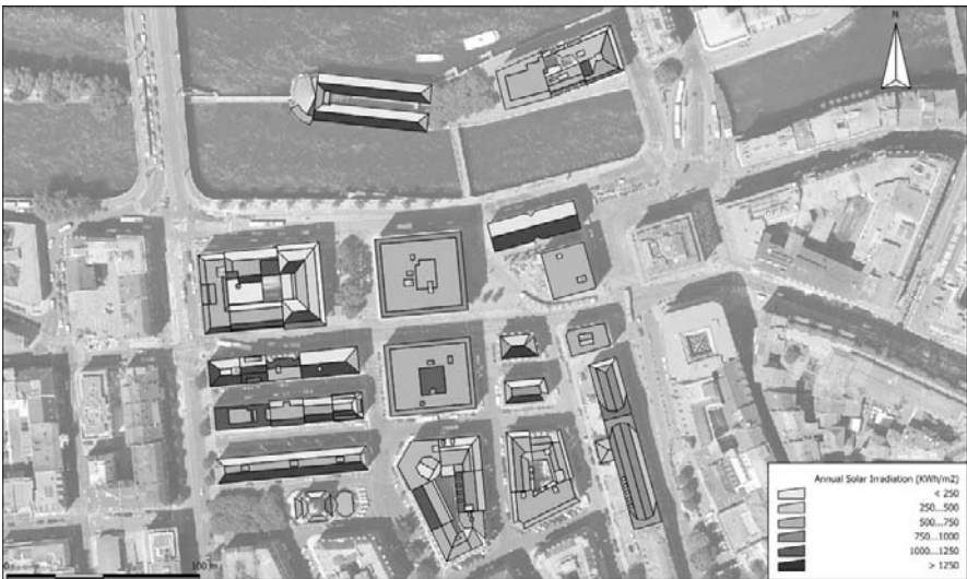
Fig. 17. Annual solar irradiance values (KWh/m 2 ) for the first pilot zone
