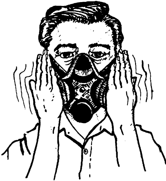
Figure 33. Negative pressure test.
