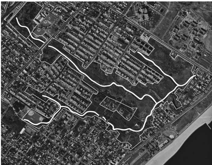
Figure 3.11 The Staten Island Bluebelt is a green infrastructure system that provides stormwater drainage for many watersheds in Staten Island, part of New York City. The system employs stormwater best management practices and created wetlands to collect, slow, treat, and release stormwater. Source USGS, Based on NYC, Department of Environmental Protection.
