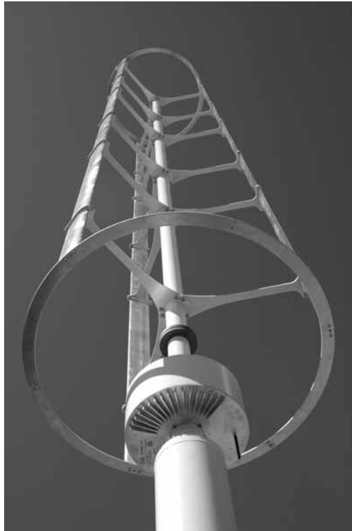
Figure 8.18 Vertical axis turbine by Mariah Power. The efficiency of the turbine is about the same as that of a turbine with a horizontal propeller. The turbine on the figure is 10 meters high with a diameter of 0.6 meters. Its power rating is 1.2 kW, and it can produce 2000 kilowatt-hours per year, Picture courtesy Mariah Power.
