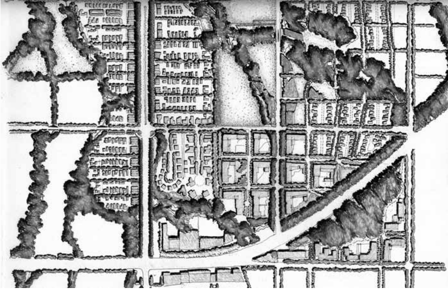
Figure 3.7 Concept design for Surrey, British Columbia, as a model sustainable urban community, clearly showing the organizing function and connectivity of the blue-green network (Courtesy Condon, 1996).
