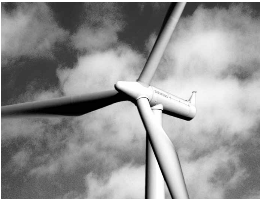
Figure 8.17 Horizontal axis wind turbine by Siemens. Large-megawatt turbines have rotor diameter up to 90 meters.
