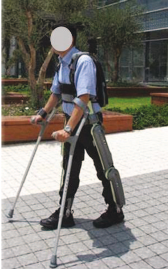
Fig. 2.6 Example of a robotized orthosis for gait restoration: a bionic walking assistance system, composed by powered leg attachments to enable paraplegics to stand upright, walk, and climb stairs
