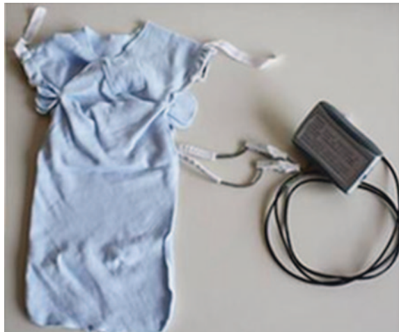
Fig. 4.2 The prototype of wearable sensor and of monitoring unit for newborns developed at the SensibiLab of the Politecnico di Milano
