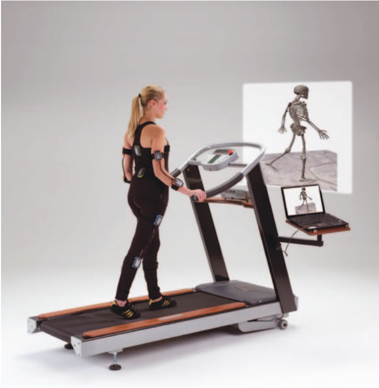
Fig. 2.9 Human movement analysis through a system of wearable inertial sensors network: example of data acquisition of the kinematics of anatomical districts and the corresponding 3-dimensional kinematic reconstruction (in the display of the figure)
