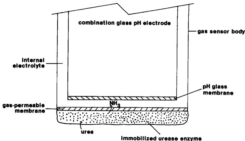
FIG. 12. Schematic of urea enzyme electrode utilizing conventional  $\text{NH}_3$  gas sensor.
