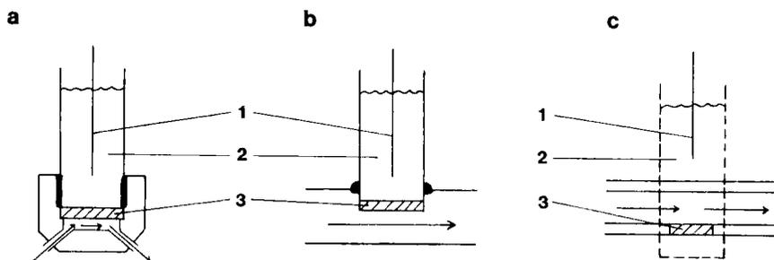
FIG. 5. Typical flow-through configurations for ISEs in clinical analyzers: (1) internal Ag/AgCl wire; (2) internal reference solution; (3) ion-selective membrane.
