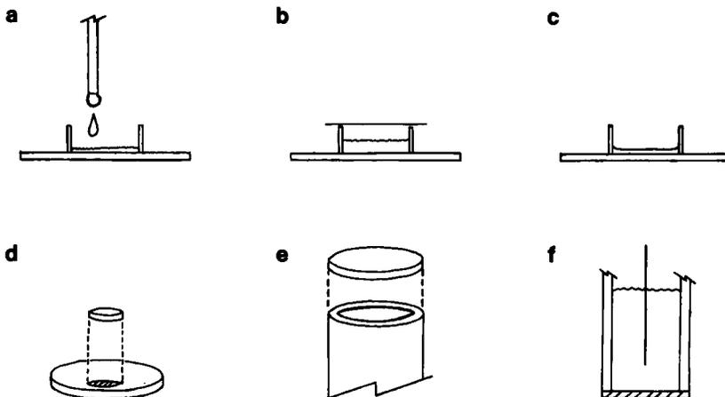
FIG. 3. Fabrication of polymer membrane ISEs: (a) dropwise addition of casting solution to glass ring resting on glass slide; (b) ring loosely covered, THF evaporates; (c) ion-selective polymeric membrane forms on the slide; (d) membrane removed from slide and small disk cut out; and (e) pasted onto a piece of PVC tubing; (f) a Ag/AgCl wire and internal reference solution complete electrode.
