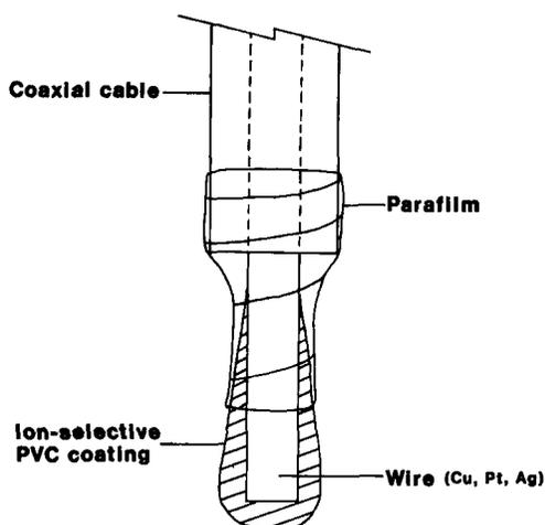
FIG. 6. Sensing tip of a coated wire ion-selective electrode.
