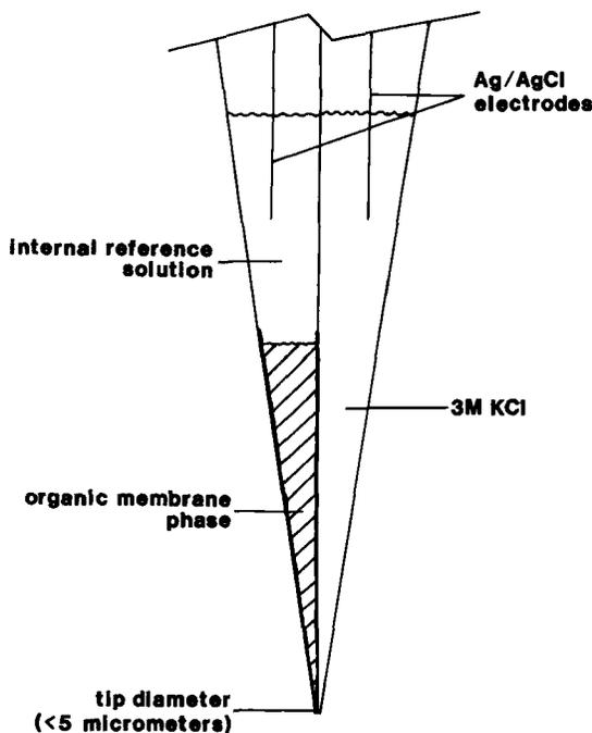
FIG. 10. Double-barrel micropipet ISE for measuring transient intracellular ion activities.
