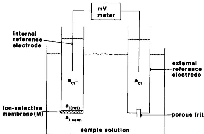
FIG. 1. Schematic of classical ISE arrangement.
