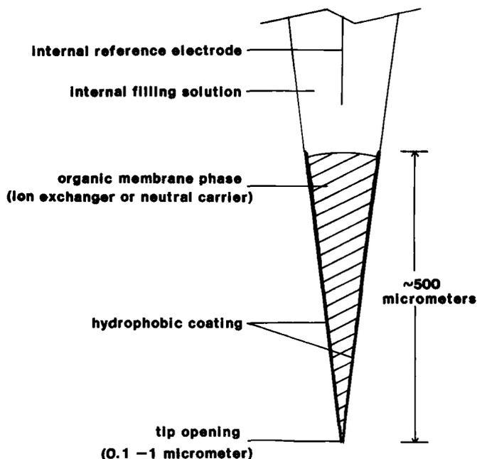
FIG. 9. Typical liquid membrane micropipet ISE.
