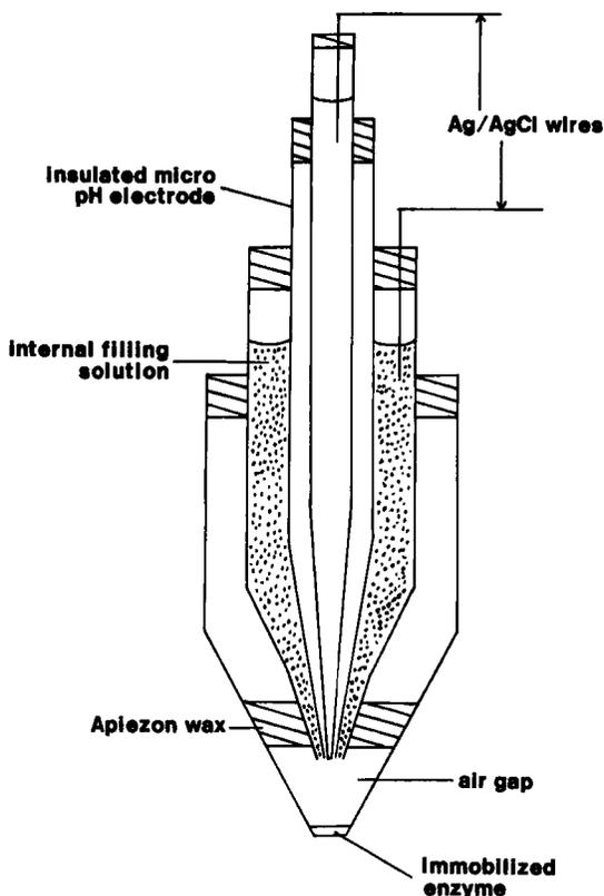
FIG. 13. Schematic diagram of microenzyme electrode [From ref. (P4). Reprinted from *Analytical Chemistry* 50. Copyright (1978) American Chemical Society.]
