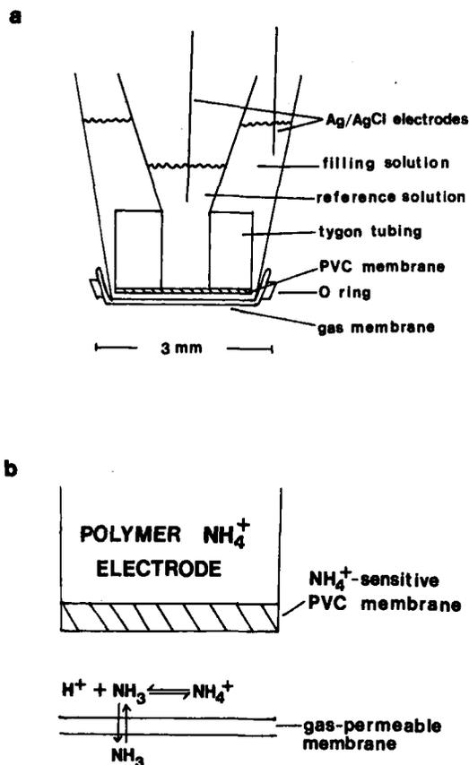
FIG. 4. (a) Schematic diagram of new polymer membrane-based  $\text{NH}_3$  gas sensor. (b) Enlargement of sensing region and the processes occurring within [From Ref. (M4). Reprinted from *Analytical Chemistry* 52. Copyright (1980) American Chemical Society.]
