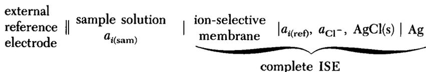
The potential of this galvanic cell containing a membrane is always measured with a high-input impedance meter as:
