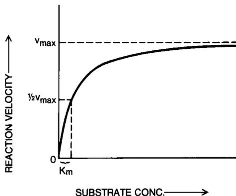
FIG. 3. Dependence of reaction velocity on substrate concentration.
