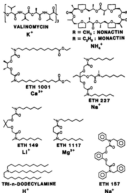
FIG. 2. Structures of some neutral carrier ionophores used in the preparation of liquid and polymer membrane ISEs [From ref. (S5) with permission. Copyright (1982), Pergamon Press.]
