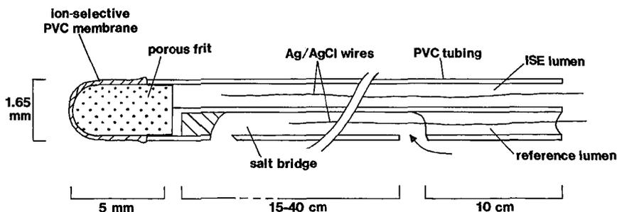
FIG. 7. Potassium-sensing catheter for *in vivo* use. [From ref. (T1) with permission.]
