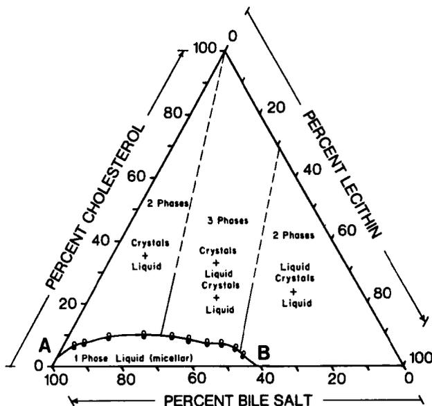
FIG. 7. Phase diagram showing the physical state of all possible combinations of cholesterol, bile salts, and lecithin (expressed as mole percent) in aqueous solutions. The line AB represents the maximum amount of cholesterol, according to Admirand and Small (A2), which can be dissolved by any mixture of bile salts and lecithin. [From ref. (A2). Reproduced from *The Journal of Clinical Investigation*, 1968, 47, by copyright permission of The American Society for Clinical Investigation.]
