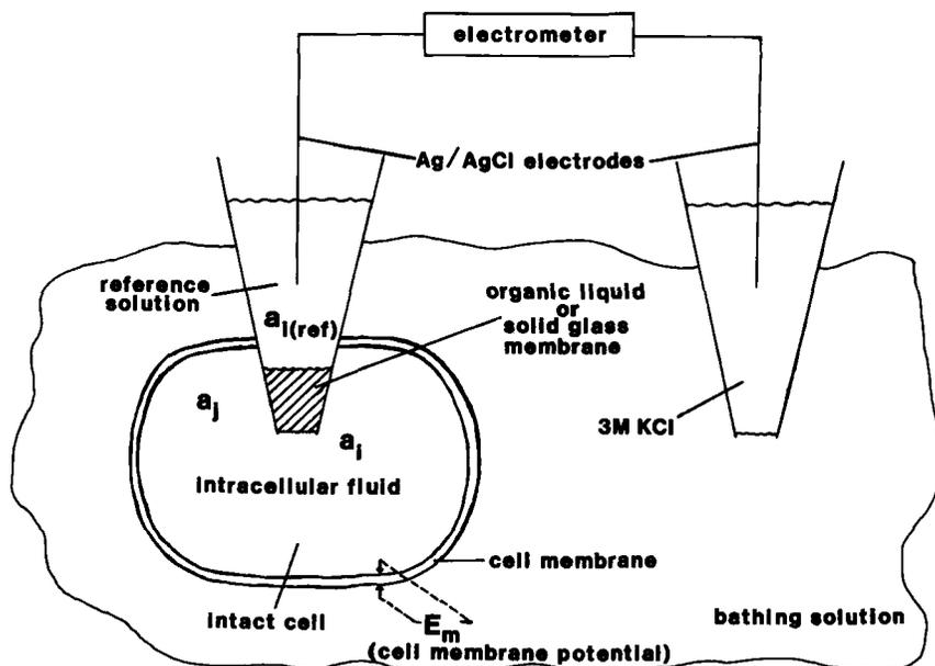
FIG. 8. Typical arrangement for intracellular ion activity measurements using micro-ISEs.
