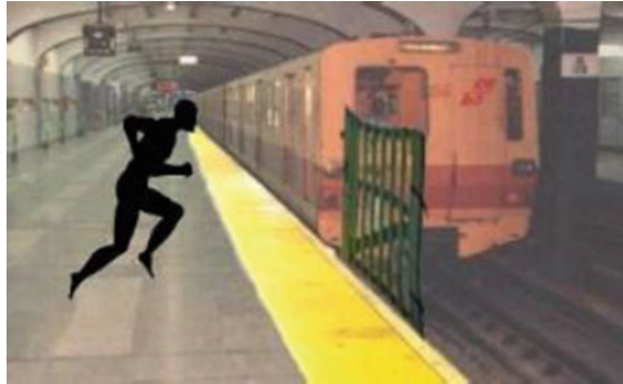
Fig. 14 Physical barrier comes up preventing the person from jumping onto the track
