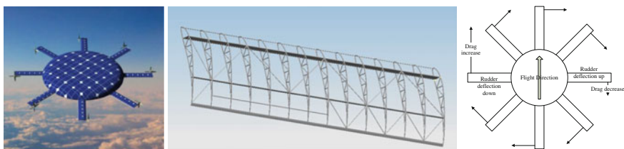
Fig. 1 The layout, structure, and flight mechanism of the aircraft
