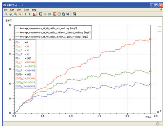
Fig. 6 Average temperature rise curves of the 40 battery monomers in the battery pack
