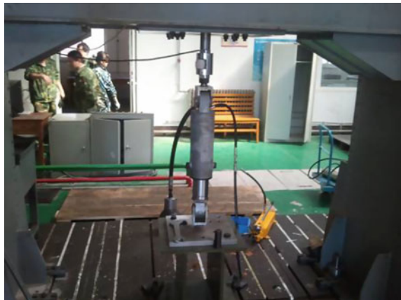
Fig. 2 Test of characteristics of oil gas spring
