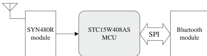
Fig. 5 Wireless remote communication circuit connection diagram
