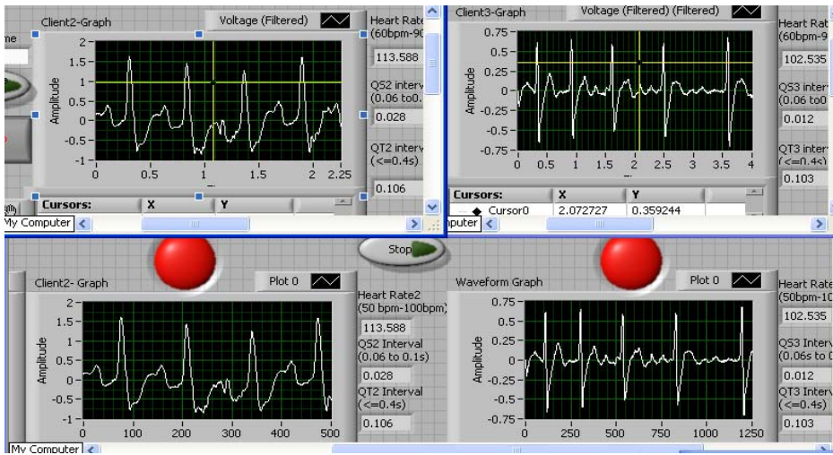
Figure 6: ECG data of patients with normal and below normal heart rate on local (top) and remote (bottom) PC (a), ECG data of patients with above normal heart rate and irregular rhythm on local (top) and remote (bottom) PC (b).
