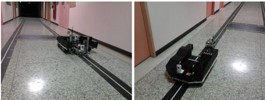
Fig. 113.8 The realistic scenes of master and slave vehicles execute the security patrol in area 1 and 2
