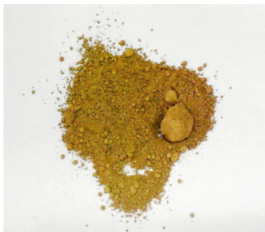
Fig. 13.1 Appearance of crude zinc dioxide
