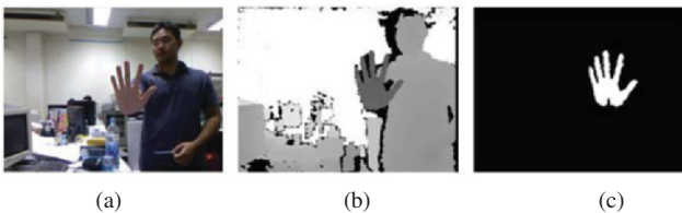
Fig. 2. Depth information: (a) complex background (b) depth image (c) hand's region.
