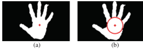
Fig. 3. Initial hand feature: (a) hand center (b) palm size.
