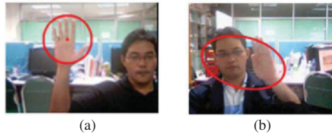
Fig. 1. Hand segmentation: (a) hand detector (b) wrong segmentation.
