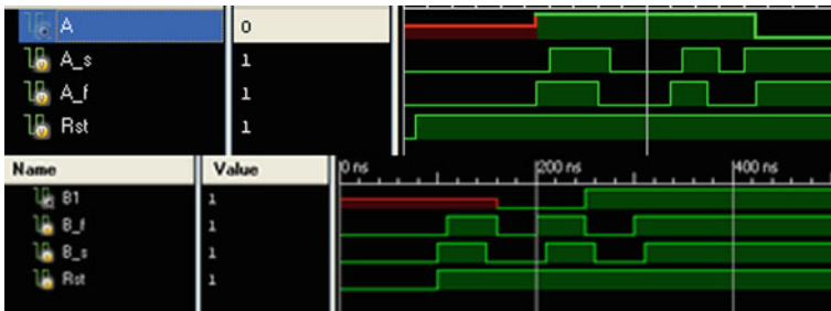
Fig. 18.9 Arbiters A and Arbiters B simulation results
