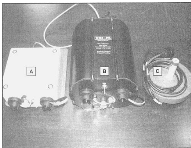
FIGURE 22 Complete cross-correlation instrument: (a) tuning circuit, (b) container incorporating demodulator and signal generator, and (c) flanged sensor unit
