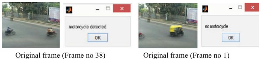
**Fig. 5** Motorcycle detection and verification using KNN classifier
