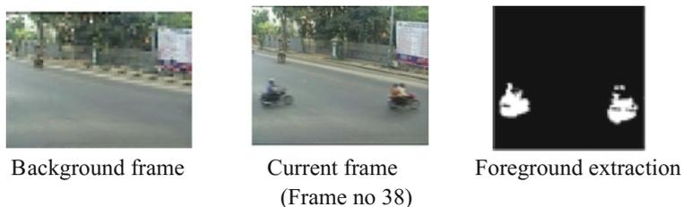
**Fig. 6** Foreground extraction using background subtraction
