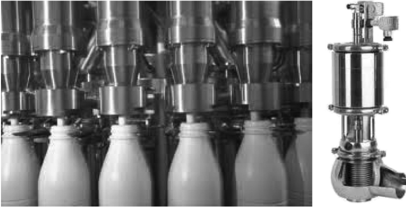
FIGURE 2.20 Constant flow valves used to fill containers.
