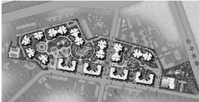
Figure 2.18. Site plan of Rover Palace ( Luofushigong ) Microdistrict designed by GZ Architects, Chengdu, 2000–2002. The microdistrict consists of 18 high-rise buildings, with a total floor space of 308,920 square metres and 1,499 apartment units.
