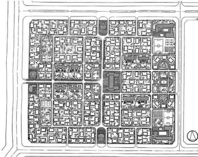
Figure 2.16. Site plan of Beiyangcun Experimental Microdistrict, Beijing, 1963. The microdistrict was planned for a population of 12,000, with 193,400 square metres of residential floor space and 37,800 square metres of service floor space.
