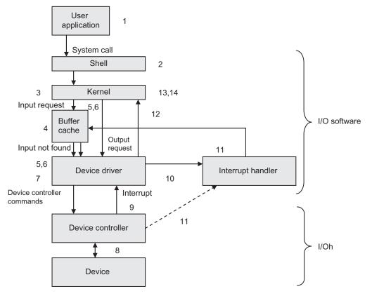
Fig. 14.4 Life cycle of an I/O request
