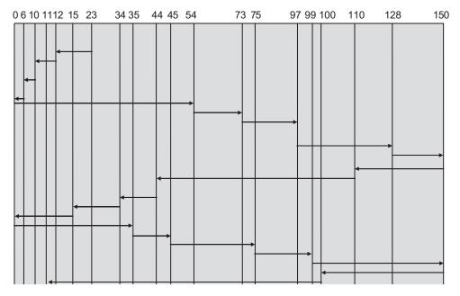
Fig. 15.12 N-SCAN disk scheduling for Example 15.7
