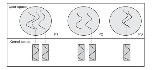
Fig. 9.8 Hybrid threads
