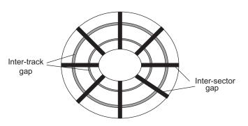
Fig. 2.12 Inter-track and inter-sector gap on the disk surface
