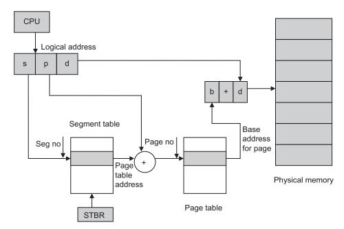
Fig. 11.23 Address translation in paged segmentation
