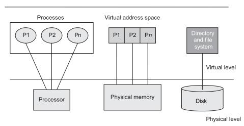
Fig. 3.4 Mapping of virtual resources to hardware Resources
