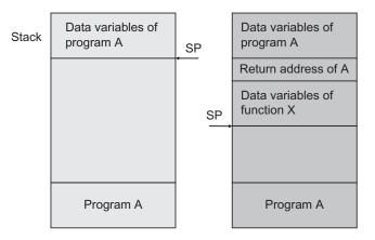
Fig. 16.2 Buffer overflow
