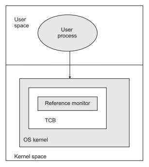
Fig. 17.10 Trusted computing base
