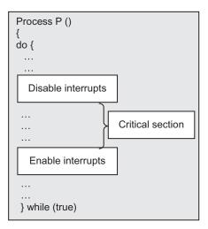
Fig. 7.40 Interrupt disabling for critical section
