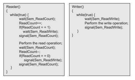
Fig. 7.15 Algorithms for reader–writer problem's solution with semaphores: readers have the priority
