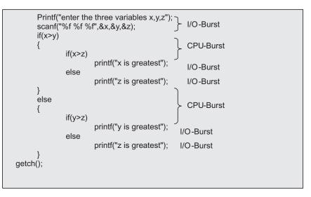
Fig. 6.1 CPU burst and I/O burst in a process
