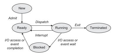
Fig. 5.4 Process state diagram
