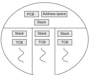
Fig. 9.4 Process's threads each with their stack and TCB
