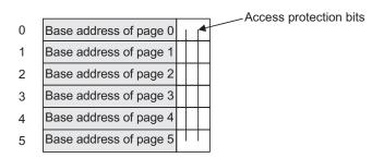
Fig. 10.20 Page table with access protection bits
