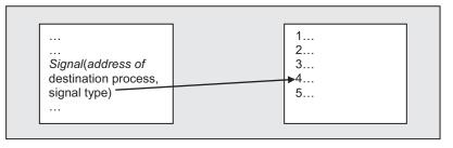
Fig. 7.37 Signal received by a process
