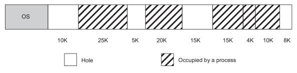
Fig. 10.13 Worst-fit allocation for Example 10.9
