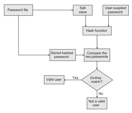
Fig. 17.8 Algorithmic flow for hash-encrypted password
