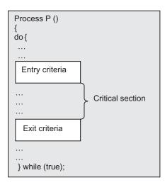
Fig. 7.3 Protocol for critical section
