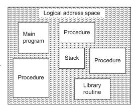
Fig. 10.28 Logical address space divided into segments
