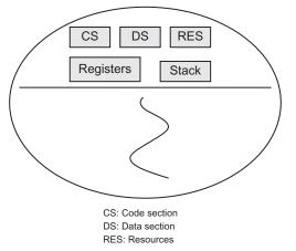
Fig. 9.1 Process as a single thread of execution
