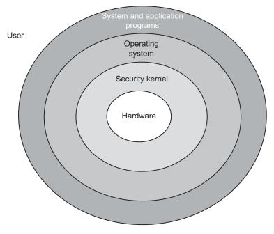
Fig. 17.9 Separate security kernel
