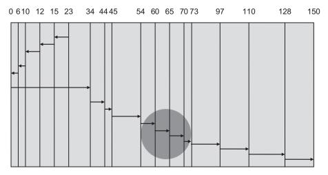
Fig. 15.5 SCAN disk scheduling for Example 15.5
