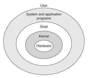
Fig. 1.14 Operating system structure with shell and kernel
