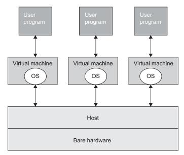
Fig. 4.9 Virtual machine architecture
