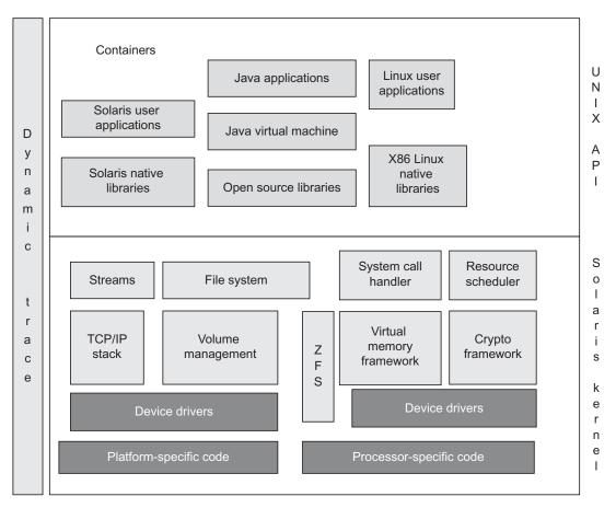
Fig. CS1.3 Architecture of Solaris 10
