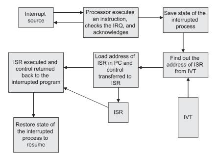
Fig. 2.2 Steps of interrupt processing
