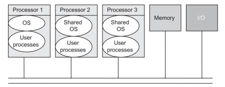
Fig. 19.3 Symmetric multi-processor configuration
