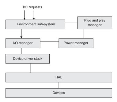
Fig. CS5.5 Input/Output management in Windows
