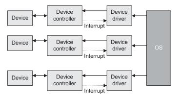
Fig. 2.4 Functioning of device driver
