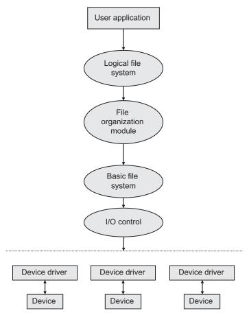
Fig. 13.1 Layered structure of the file system
