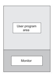
Fig. 1.4 Memory structure consisting of resident monitor
