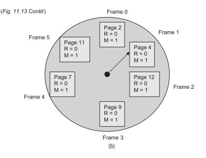
advanced to the next frame. Coincidently, all the frames in the queue have R and M bits set as 1. Therefore, one round of the algorithm does not find any page to be replaced. However, in the next round, all pages have R bits reset to 0. Therefore, the first page, that is, Page number 4, can be chosen for the replacement as shown in Fig. 11.13(b).
