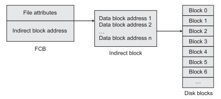
Fig. 13.5 File mapping through indirect block
