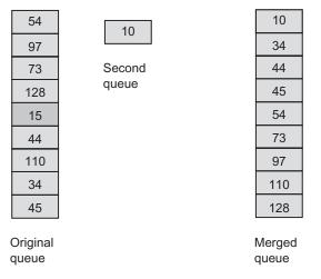
Fig. 15.8 F-SCAN first pass for Example 15.7
