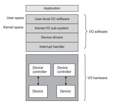
Fig. 14.1 Layered structure of I/O
