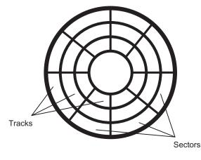
**Fig. 2.10** Track and sectors on a disk platter surface
