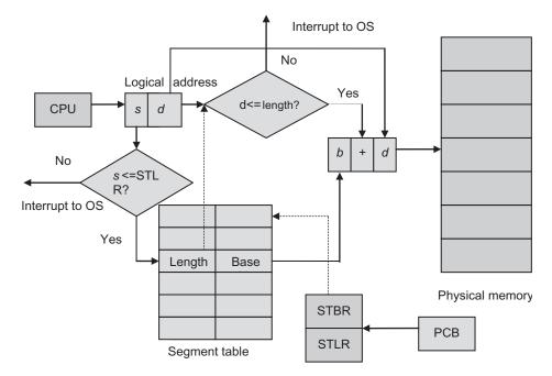
Fig. 10.31 Hardware requirements for address translation in segmentation
