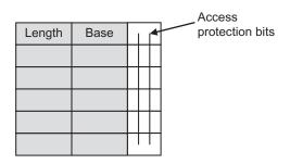
Fig. 10.32 Segment table with access protection bits
