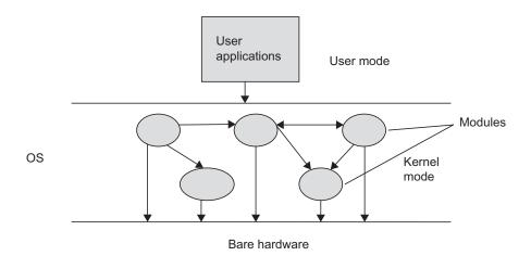
Fig. 4.6 Monolithic architecture
