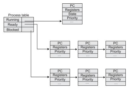
Fig. 5.10 Separate queues for different states of the processes
