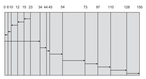
Fig. 15.4 SCAN disk scheduling for Example 15.4
