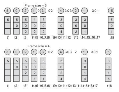
Here, in optimal algorithm, at every instant of time, the page\_set in execution with page-frame size = 3 is the subset of the page\_set in execution with page-frame size = 4. Thus, this algorithm satisfies the stack property.
