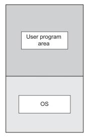
In older systems, memory allocation is done by allocating a single contiguous area in memory to the processes. When there was multi-programming or a multi-user system, memory was divided into two partitions, - one for the OS, and the other for the user process (see Fig. 10.4). The user process in its partition has a single contiguous region of memory.
