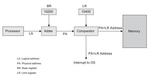
Fig. 10.3 Memory mapping using base and limit registers
