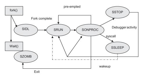
Fig. CS2.6 Process state transition diagram
