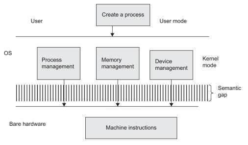
Fig. 4.7 Semantic gap between the OS and hardware
