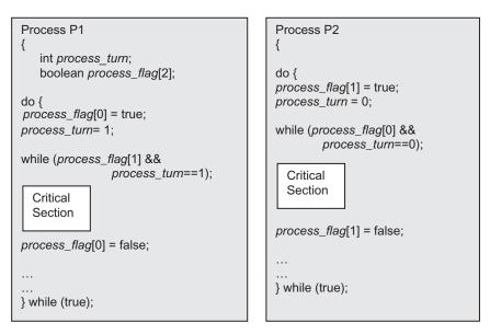
Fig. 7.8 Peterson's solution for two-process synchronization
