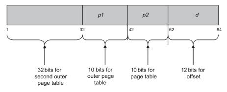
Fig. 10.26 64-bit Logical address corresponding to three-level page table structure
