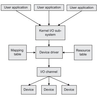
Fig. 14.2 Device driver interface
