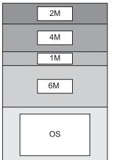
Fig. 10.7 Fixed unequal-sized partitioning-based contiguous memory allocation
