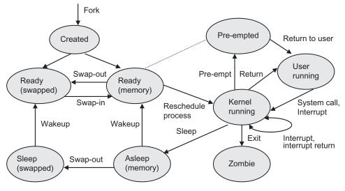
Fig. CS2.1 Process state transition diagram
