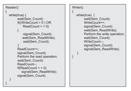
Fig. 7.17 Algorithms for reader-writer problem's solution with semaphores: No priority
