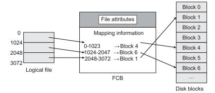
Fig. 13.4 File mapping through FCB
