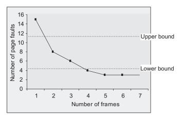
Fig. 11.22 Page fault frequency
