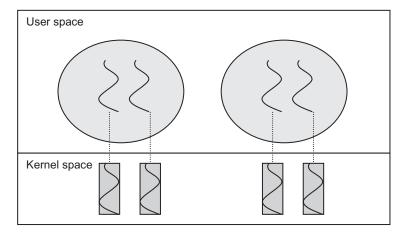
Fig. 9.7 One-to-one mapping in kernel threads
