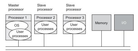
Fig. 19.2 Master-Slave multi-processor configuration
