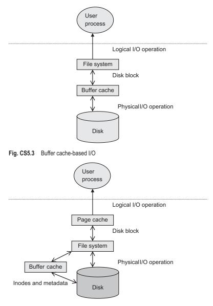
Fig. CS5.4 Page cache-based I/O
