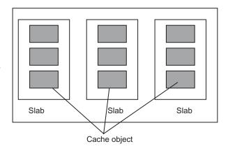
Fig. CS3.6 Components of a slab allocator
