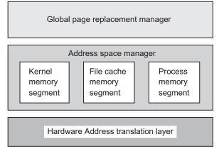
Fig. CS3.3 Virtual memory management in Solaris
