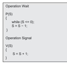
Fig. 7.9 Wait and signal operation in a semaphore
