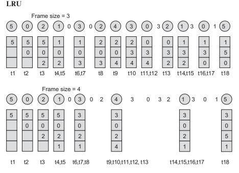
Here, in LRU algorithm, at every instant of time, the page\_set in execution with page-frame size = 3 is the subset of the page\_set in execution with page-frame size = 4. Thus, this algorithm satisfies the stack property.
