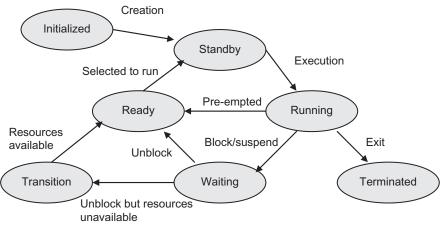
Fig. CS2.8 Thread state
