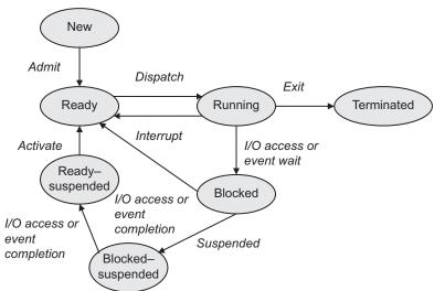
Fig. 5.5 Process state diagram with suspended states
