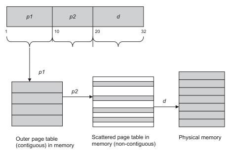
Fig. 10.25 Address translation using two-level page table structure
