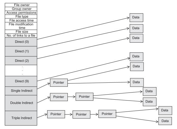
Fig. CS4.1 File allocation in UNIX
