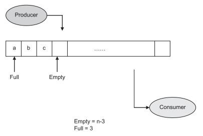
Fig. 7.13 Producer–consumer problem's solution with semaphores
