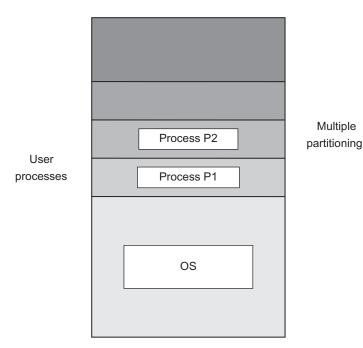
Fig. 10.5 Multiple partitioning of memory
