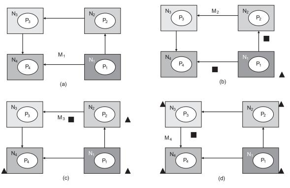
Fig. 18.6 Chandy–Lamport consistent state recording algorithm Example 18.2
