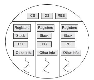
Fig. 9.3 A process divided into three threads of execution
