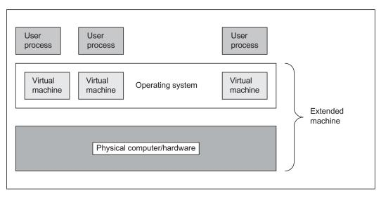
Fig. 1.13 Operating system as a virtual machine manager
