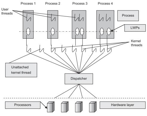
Fig. CS2.5 Multi-threaded process model
