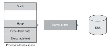
Fig. CS5.1 File I/O with kernel buffer
