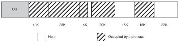
Fig. 10.12 Best-fit allocation for Example 10.9
