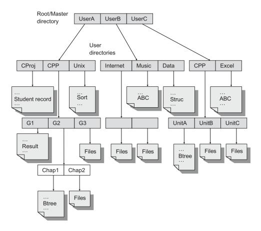
The tree-directory structure, shown above, consists of files having identical names. But the files can be easily accessed using pathnames. Both user A and user C consist of a file named 'Btree'. The files, however, can be distinguished and accessed using the following path names:
