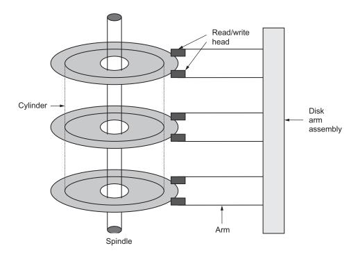
Fig. 2.11 Physical structure of a disk
