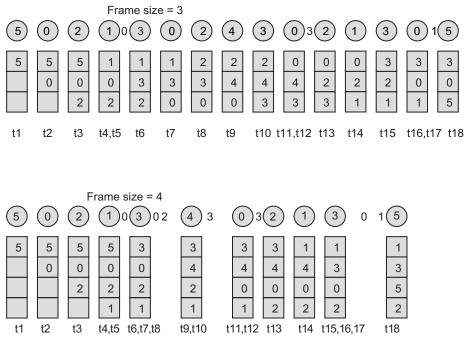
In FIFO, at time instants t9 and t18, the page\_set in execution with page-frame size = 3 is not the subset of page\_set in execution with page-frame size = 4. Thus, this algorithm does not satisfy the stack property.
