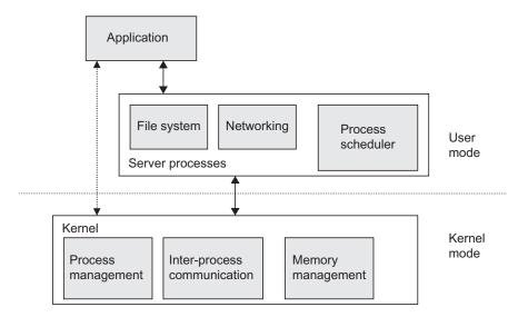
Fig. 4.11 Microkernel architecture
