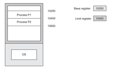
Fig. 10.2 Relocation with base and limit register
