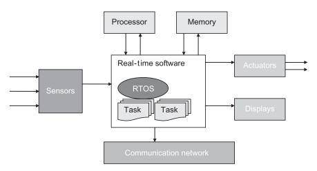
Fig. 20.2 Structure of a real-time system
