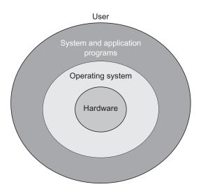
(see Fig. 1.2). This software is known as *operating system* (OS) and is the answer to all the questions asked earlier. The OS starts functioning right from the moment we switch on the computer system and continues till we shut down the system.
