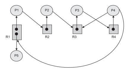
In this scenario, processes P1, P2, P3, and P4 are holding one resource each, and requesting for one more resource, which is held by the next process. From the RAG drawn above, it can be seen that there is a cycle, in the form of circular wait in the graph, thereby, causing a deadlock situation.
