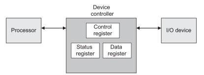
Fig. 2.3 Device controller registers
