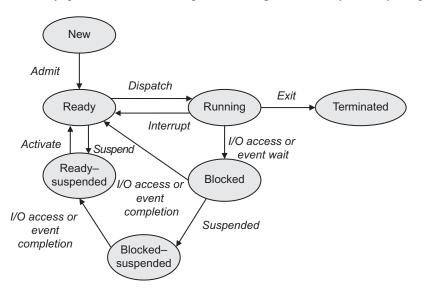
Fig. 5.6 Process state diagram with ready to ready-suspended transition
