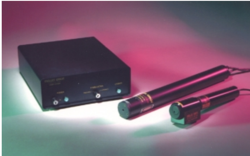
Fig. 6-1 Modern He-Ne laser manufactured by Melles Griot. (Photo, courtesy of Melles Griot).
