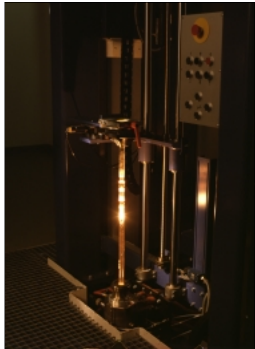
Fig. 3-12 Fiber drawing - top of the tower
