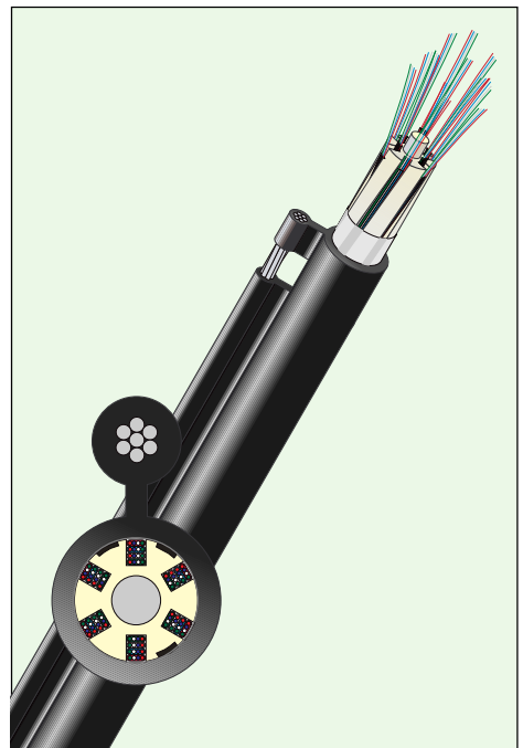
Fig. 5-36 With a steel suspension strand, optical fiber cable can be suspended in spans of 50 - 70 m. The cable illustrated is GASLCV.
