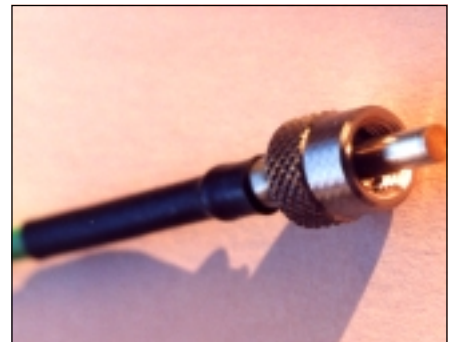
Fig. 8-26 LME connector, one of the first connectors for optical fiber cable.
