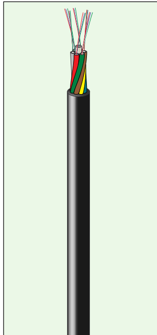
Fig. 5-39 Cable to be wrapped around ground wire or phase line "Skywrap"
