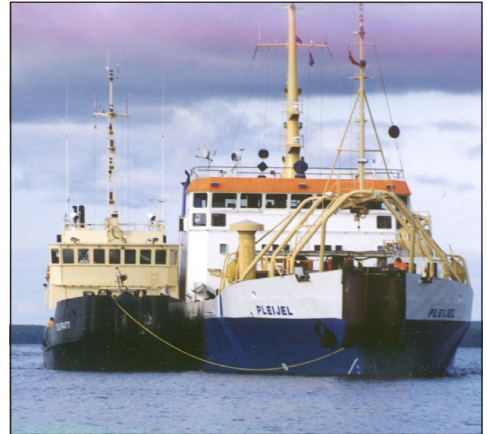
Fig. 11-28 Especially equipped vessel for laying submarine cable (Telia's Pleijel).
