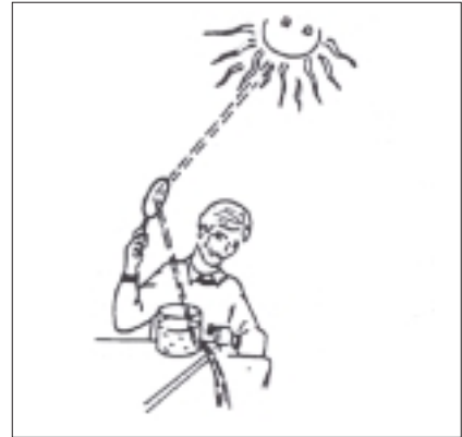
Fig. 1-4 By demonstrating that light could travel along a bent water jet, the principle of optical transmission in light conductors was established.
