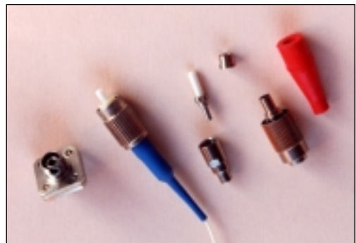
Fig. 8-28 FC-FC/PC connector in bits and pieces. To the left is the mounting bushing to be fitted in the ODF box.
