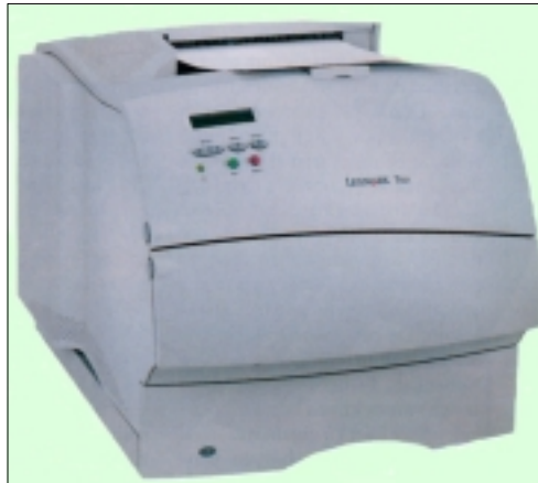
Fig. 6-5 Laser printers have revolutionized the graphics industry. Modern laser printers have a resolution of over 1200 dpi.
