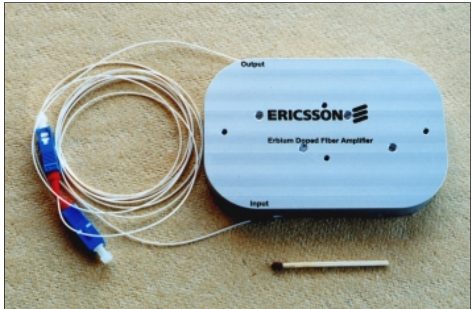
Fig. 12-14 EDFA with a size comparing match.
