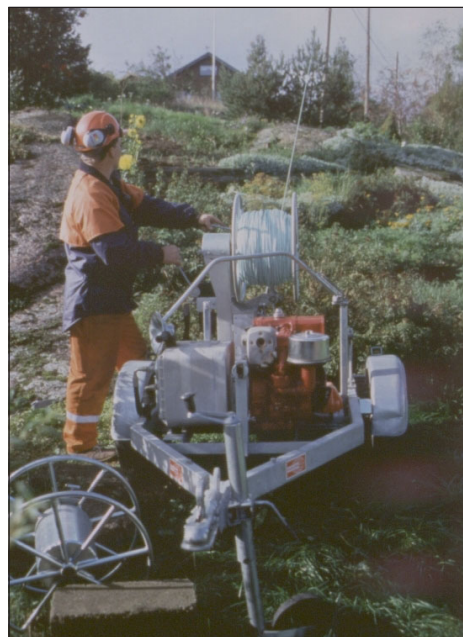
Fig. 11-24 Gasoline powered winch for installing aerial cable. Photo: Courtesy of Sahlins, Sweden.
