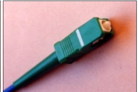
Fig. 8-31 SC connector for analog transmissions, the ferrule is polished with 8 degree angle. These connectors are generally in green.
