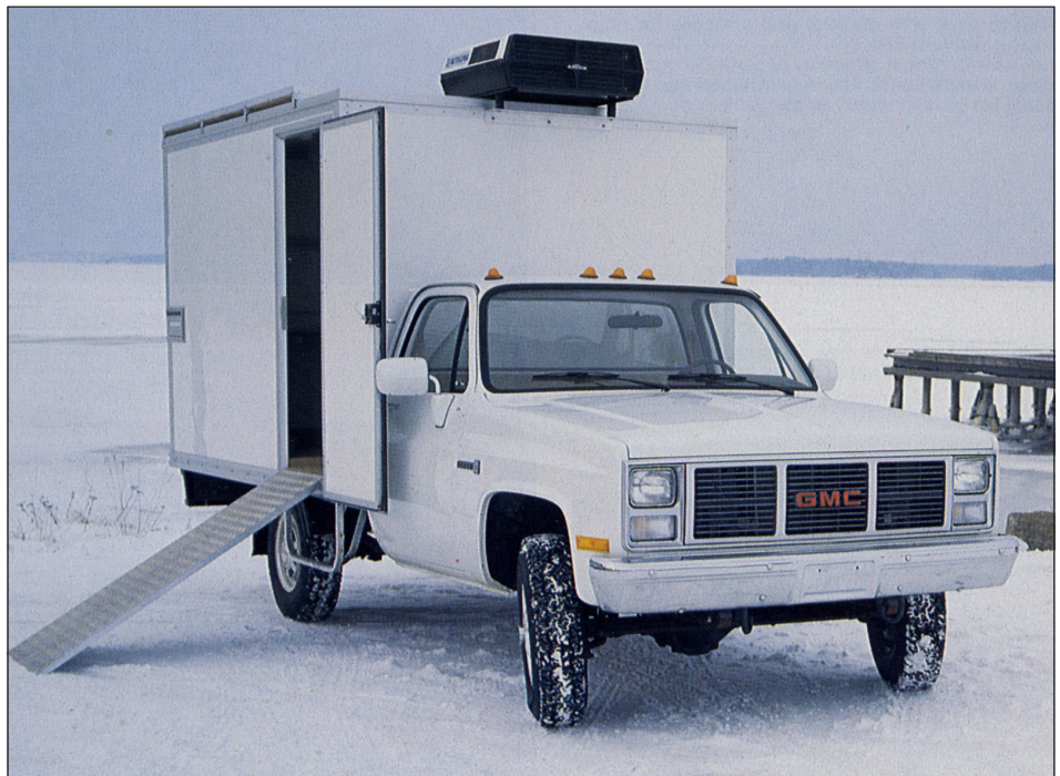
Fig. 11-42 Specially equipped vehicle for splicing optical fiber cable in the field.
