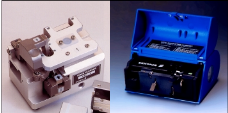
Fig. 8-15 The quality of the fiber cutter used can often determine the performance of a splice. A fiber cutter of high quality cuts the fiber rapidly and safely at a 90° angle, without deforming the cutting surface. The cutters above are from Sumitomo (left) and Ericsson (right). The Sumitomo cutter also cuts fiber ribbon.
