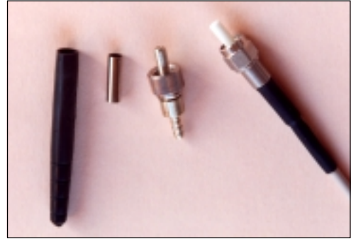
Fig. 8-27 The SMA connector became an international standard. The figure shows one connector with ceramical ferrule and one with a metallic ferrule.
