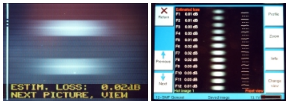
Fig. 8-17 Two electronically scanned images. The picture to the left shows a picture taken during the fusion process of a single fiber and the picture to the right shows the same for a 12-fiber ribbon splicer. The fiber core is visible as a light-colored stripe in the middle of the fiber (left picture only). This picture shows also the fiber in both horizontal and vertical direction. The picture with the 12-fiber ribbon is only in vertical direction.
