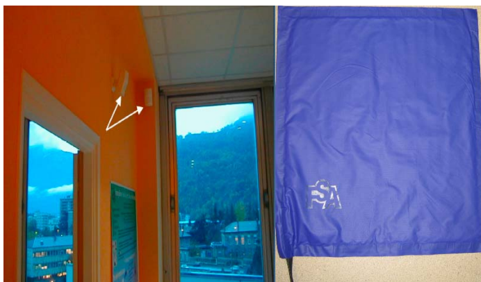
Fig. 1. Infrared (arrows) for localizing dependent people in a health smart home (left) & pressure sensors (right: FSA Seat 32/63 pressure mapping system, Vista Medical Ltd)
