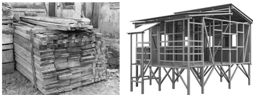
Fig. 14.4 Photograph of a house ‘kit’ (a set of materials for its construction), as well as a three-dimensional model of a recurrent typology of housing, showing its wooden structure and walling. Source Photograph by the author (2012). Model: survey and modelling by the author, rendering by Hugo Machado da Silva (Fernandes 2015)
