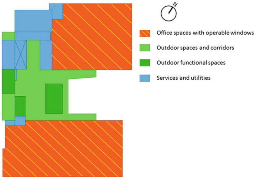
Fig. 3.2 Schematic diagram of building layout at upper floors of IBR HQ building (The Authors, adapted from Cao et al. 2014)
