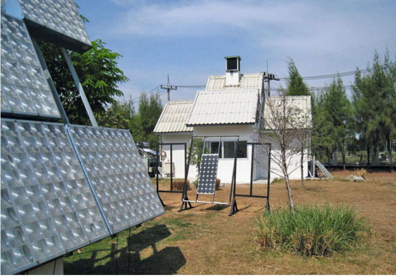
Fig. 5.3 Test house for energy, indoor comfort, ventilation and daylighting, JGSEE Thailand (Source: Chris Butters)
