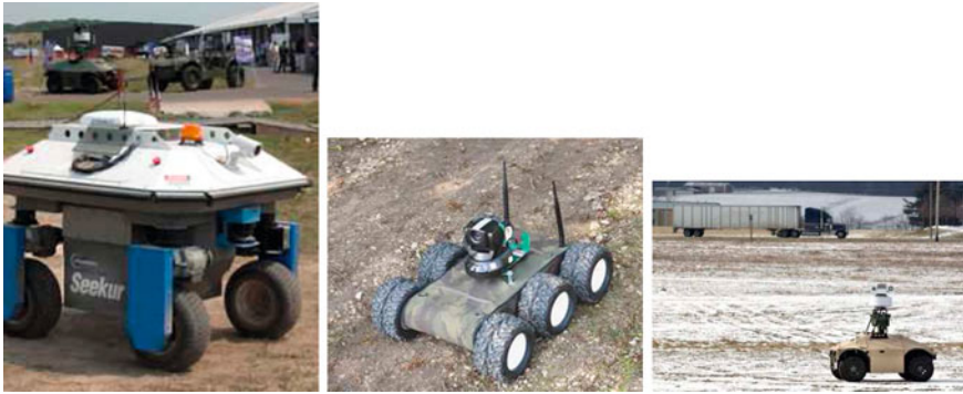
Fig. 1.3 Surveillance vehicles: 1. Seekur UGV from MobileRobots Inc, 2. \mu Trooper from Thales, and 3. MDARS from general dynamics
