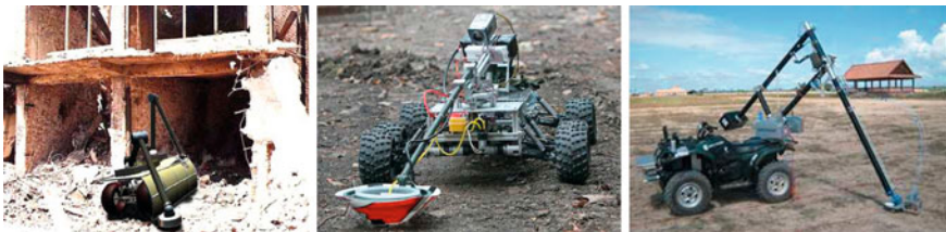
Fig. 1.4 Humanitarian demining vehicles: 1. Buggy-robot from Hirose and Fukushima laboratory, 2. Humi from TU Wien, and 3. Gryphon-III with field arm from Hirose and Fukushima laboratory
