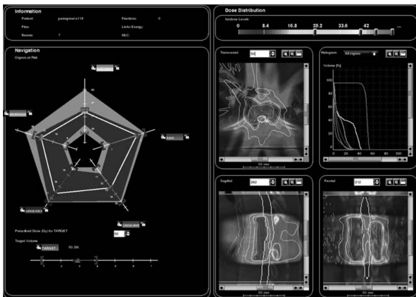
Fig. 5.19. The navigation screen. The “star” on the left-hand side shows the active and inactive planning horizon and the current solution. On the right the dose visualization and the dose-volume histogram for the current solution are shown.
