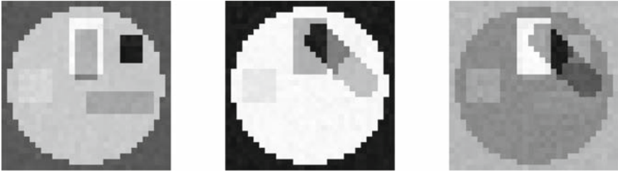
Fig. 8.10. Example: poorly recovered source signals using ICA. The signal-to-noise ratio between the original sources (Figure 8.6) and the recoveries is very low with 3.3, 13 and 12 dB after permutation and normalization.
