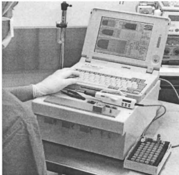
Fig. 7. The ROTEG Coagulation Analyzer: a new thrombelastographic analyzer suitable for use in the OR or ICU. Four tests can be assessed in parallel and are shown on the computer display
