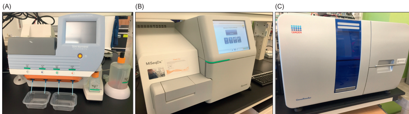
FIGURE 4.3 The desktop DNA sequencer. Desktop sequencers are a favorite of many molecular diagnostic laboratories due to the small footprint, assay adaptability, and sequencing capacity. These sequencers have the capacity to screen and diagnosis genetic disease through gene specific or gene panel tests, identify low-level variation in solid tumors through “hotspot” gene panel testing, and sequence the clinical exome. The most common instruments found in today’s molecular diagnostics laboratory’s are (A) the IonTorrent PGM (Thermo Fisher), (B) the MiSeqDx (Illumina) which is currently the only FDA-approved sequencer, and (C) the GeneReader NGS system (Qiagen) which is the only fully automated desktop sequencer released in late 2015.
