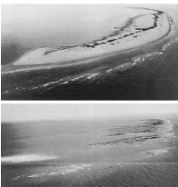
Fig. 18.10 Raccoon Island, Louisiana, USA, before (top) and after (bottom) the passage of Hurricane Andrew in August 1992. The detached barrier island was originally ca 5 km long but was heavily scoured, shortened and flattened by storm waves and washover transport. (From Eos, 1992.)
