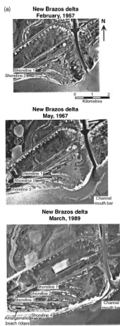
Fig. 17.22 (a) Scaled and orientated aerial photos of the New Brazos delta illustrating delta progradation. Following each large flood a new ridge/trough pair was preserved in the western delta. (After Rodrigues et al. , 2000.) (b) Scaled aerial photos of the New Brazos delta illustrating the progradation event that resulted from the 1965 flood. (Modified by Rodrigues et al. , 2000.)
