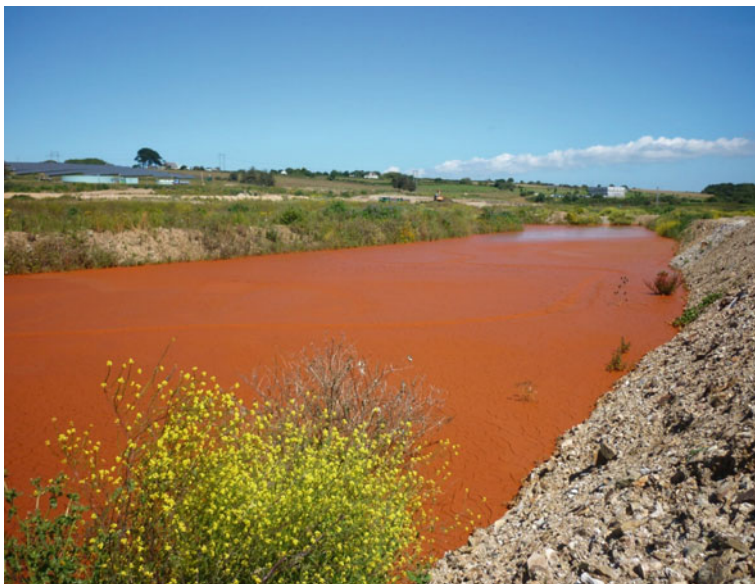
Fig. 6.38 Operating paddock for minewater sludge on surface of CVTD, UK
