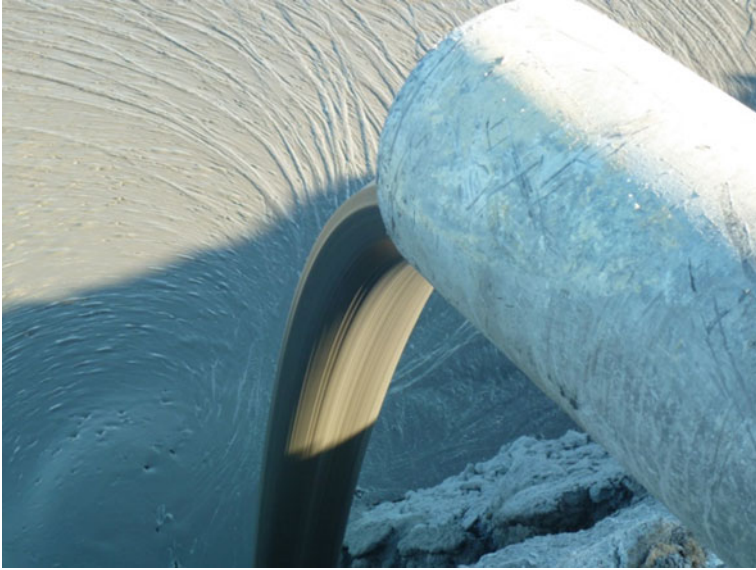
Fig. 6.29 Typical thickened discharge
