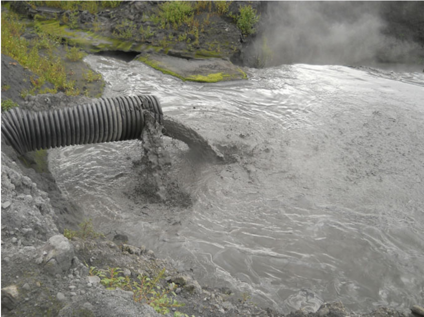
Fig. 8.1 Hydraulic disposal of fly-ash
