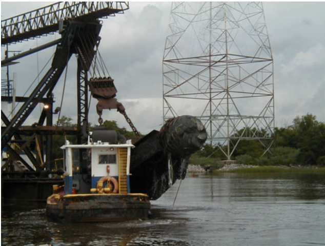
Dredging, Figure 2 Cutterhead tool lifted clear of the water.
