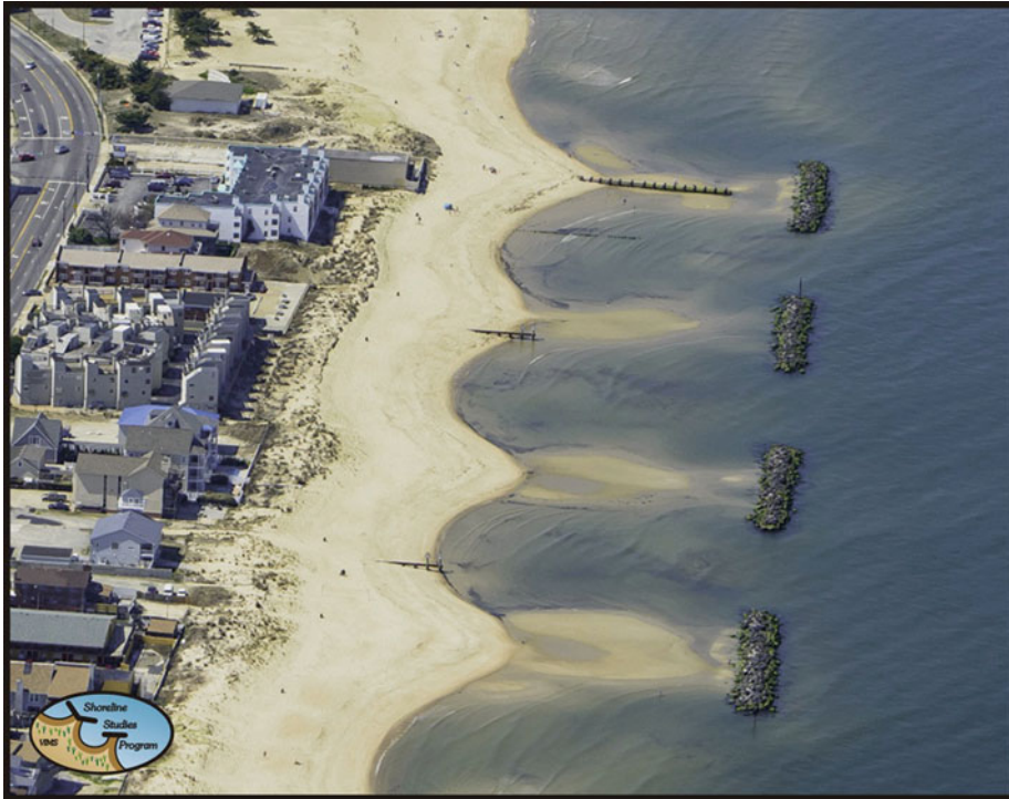
Shore Protection, Figure 5 Detached breakwaters that have a shore salient behind the structures. These structures are located in an area with a strong sand transport system and are designed to allow the sediment to move through the system to downdrift shores.
