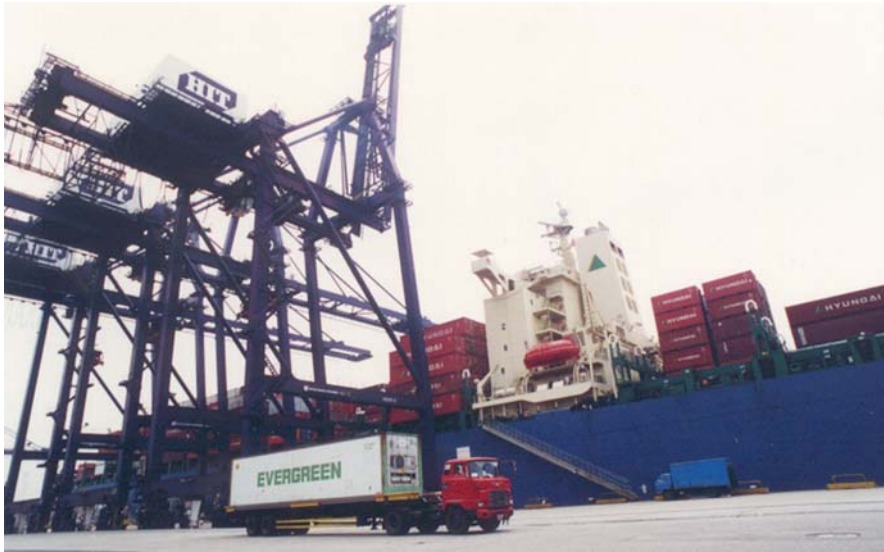
Fig. 3.4 A docked vessel and QCs unloading inbound containers from it and loading outbound containers into it. Also see a TIT (terminal's internal truck) that transports containers between the berth and the SY
