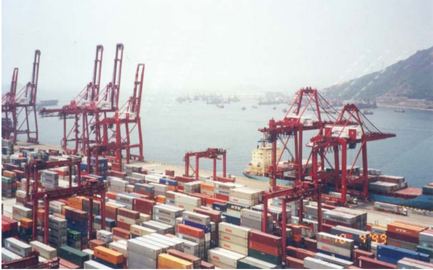
Fig. 3.2 Containers in temporary storage at the storage yard (SY). At water's edge, see quay cranes (QC) unloading, loading containers from, into vessels. In SY, see yard cranes (YC) that store and retrieve containers from storage
