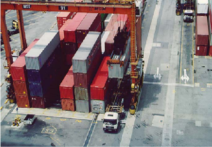
Fig. 3.3 Six rows of stored containers and seventh ( rightmost ) lane for truck passing in a storage block. You can see the RTGC lowering a retrieved container from storage onto a truck
