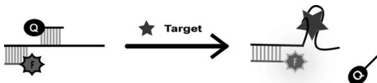
Fig. 5 Structure-switching approach. Target ( star shape ) promotes structure-switching of an aptamer from a DNA–DNA duplex ( left ) to a DNA–target complex ( right ). The dissociation of quencher-labeled DNA strand (QDNA) from the aptamer is accompanied with an increase of fluorescence signal. F and Q denote fluorophore and quencher, respectively
