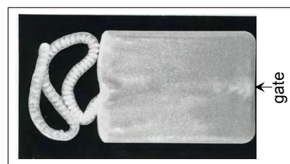
Figure 3.10 Short-shot moulding showing jetting (source: Akay (1992))
