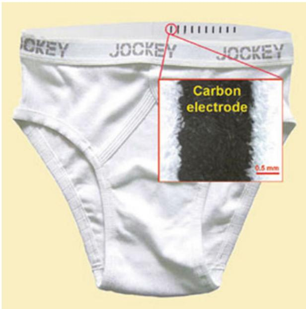
**Fig. 4.3** The proposed on-body noninvasive textile-based sensing incorporated within men's briefs. Reproduced from [23] with permission from the Royal Society of Chemistry
