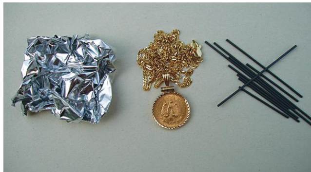
FIGURE 2-5 Examples of elements. Aluminum foil is 98.5% aluminum. Twenty-four carat gold is 99.9% gold. Graphite is 100% carbon.
