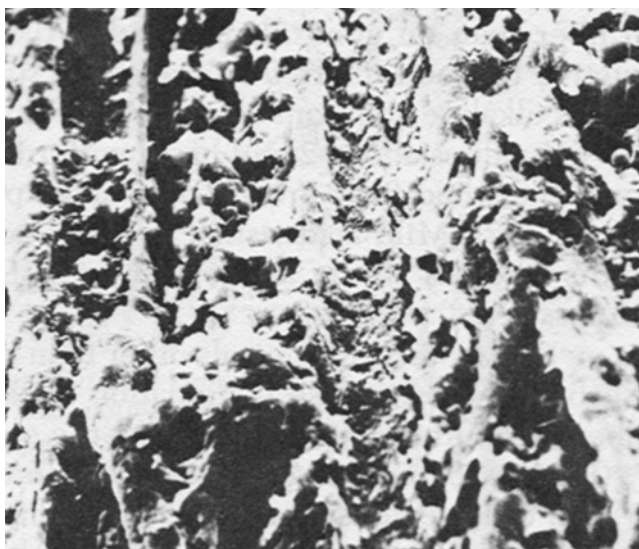
FIGURE 11.18 Scanning electron micrograph of sodium chloride in southern pine cell ( \times 400 ).
