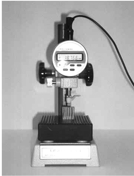
FIGURE 4.5 Measuring wood swelling using a flat-bed micrometer.
