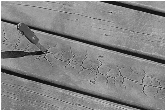
FIGURE 7.5 Cross-grain checking in juvenile wood.
