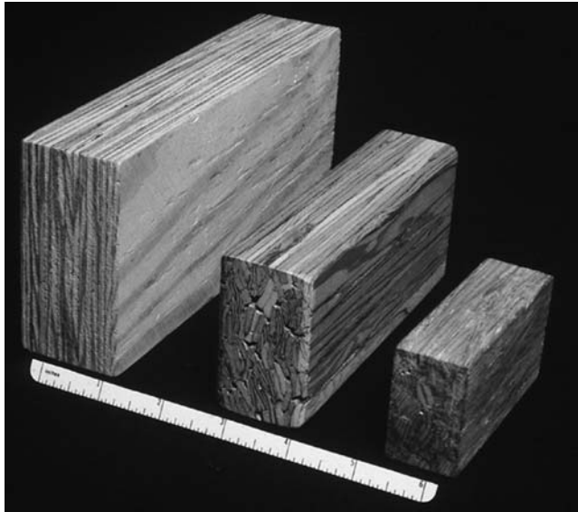
FIGURE 10.5 Three types of structural composite lumber (SCL). Left—Oriented strand lumber (OSL), center—Parallel strand lumber (PSL), right—Laminated veneer lumber (LVL).
