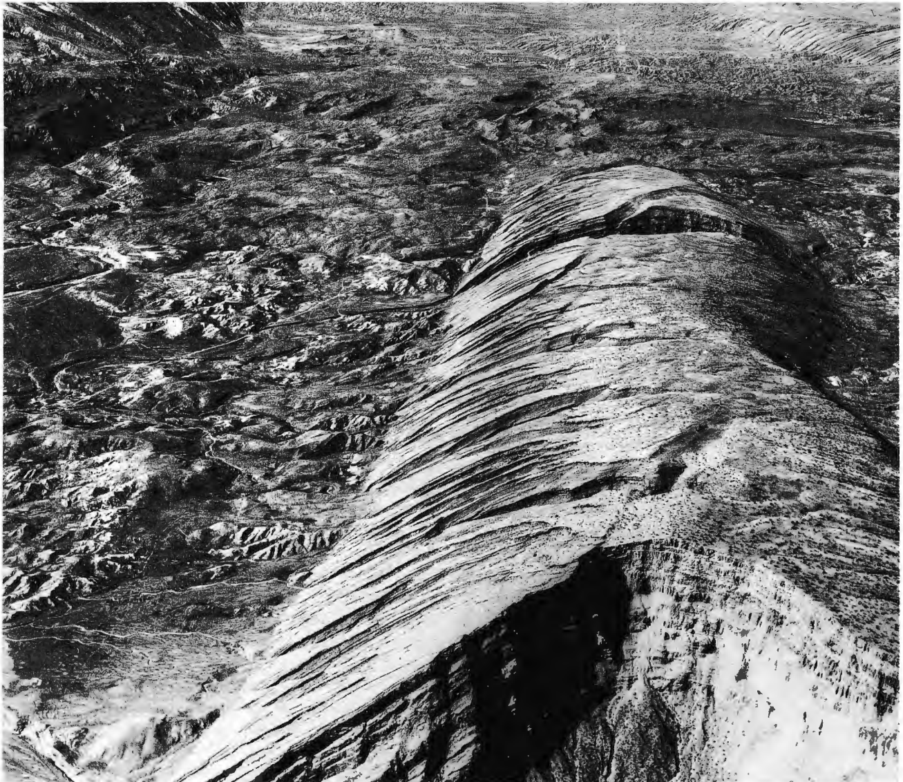
Fig. 3.18 Limb of the Saidmarreh anticline, southern Zagros Mountains, Iran. This plunging anticline is experiencing active uplift and although breached by a major stream has retained much of its primary form. (Photo courtesy Aerofilms Ltd.)
