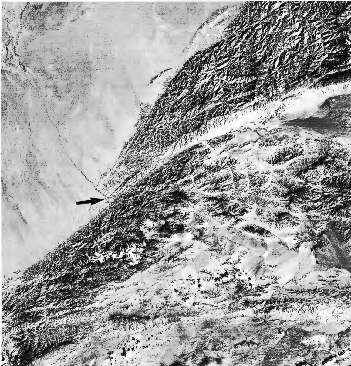
Fig. 3.25 Landsat image of the Altyn Tagh Fault north of the Kunlun Shan Mountains. Left-lateral movement along the fault is evident from the offsetting of stream channels which cross it (arrowed). (Image courtesy N. M. Short.)
