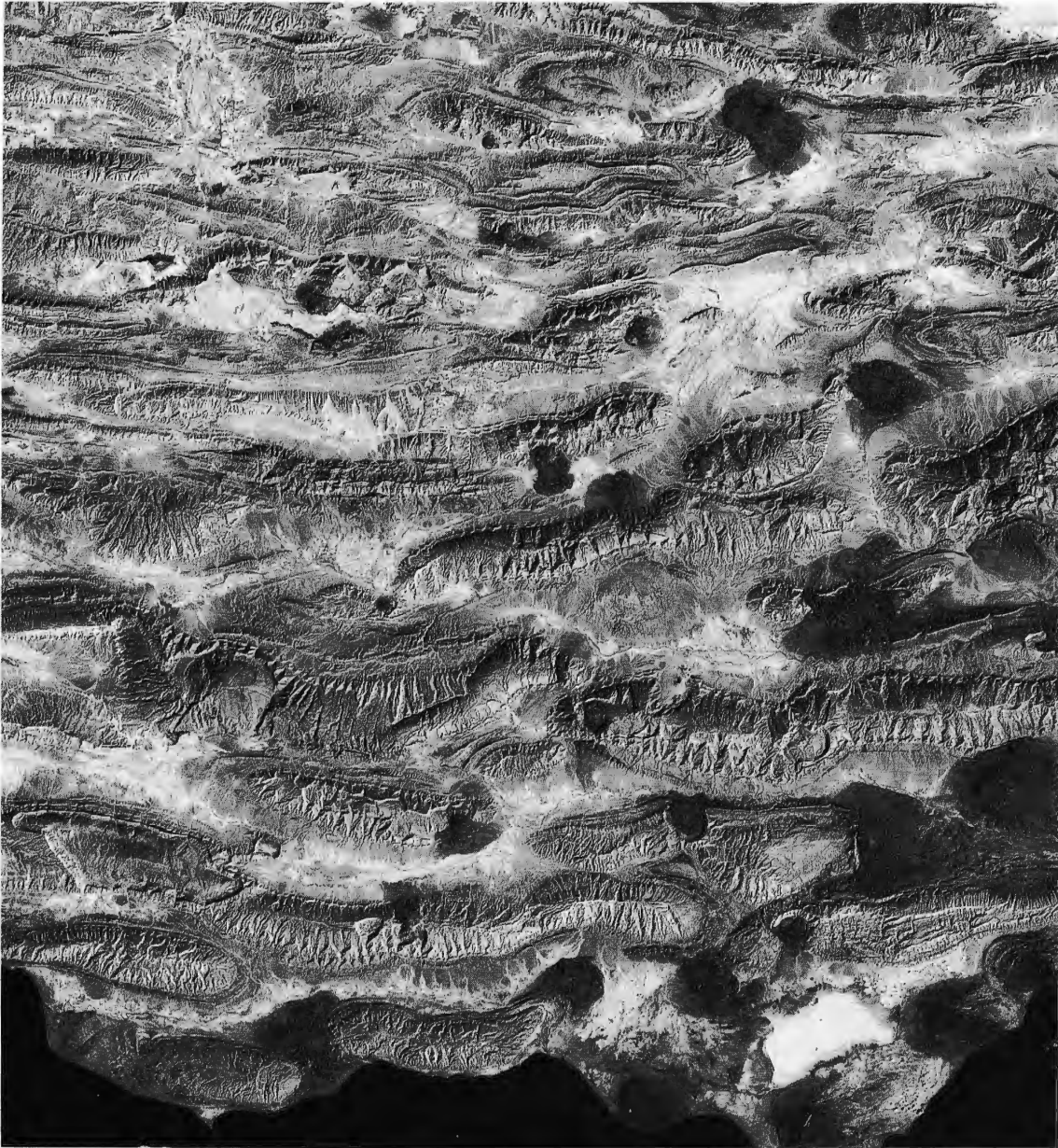
Fig. 3.17 Landsat scene of part of the southern Zagros Mountains, Iran. Sediments of Mesozoic and Early Cenozoic age laid down on a continental shelf have been folded into a succession of plunging anticlines as a result of compression arising from intercontinental collision. The sediments contain thick salt beds which in places have intruded overlying strata as a result of their lower density and reached the surface to form salt fountains up to 1 km high (small, dark patches on image) The salt spreads under its own weight at rates of a few \text{m a}^{-1} forming salt flows. (Image courtesy N. M. Short.)
