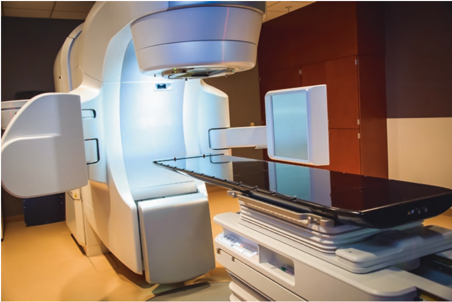
Fig. 4.5 Modern linear accelerator with imaging arms extended (OBI). They are capable of obtaining X-rays vital for patient setup. By rotating 360°, the imaging arms are capable of producing a CT image set
