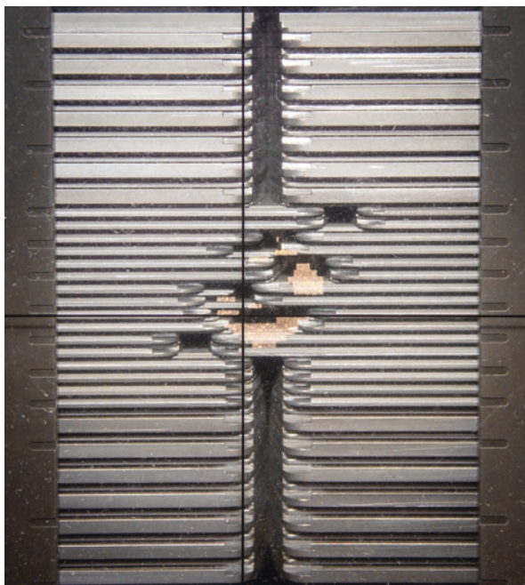
Fig. 4.3 Multi-leaf collimator. Multiple small leaves conform to desired shape, or move during treatment delivery to create a modulated field
