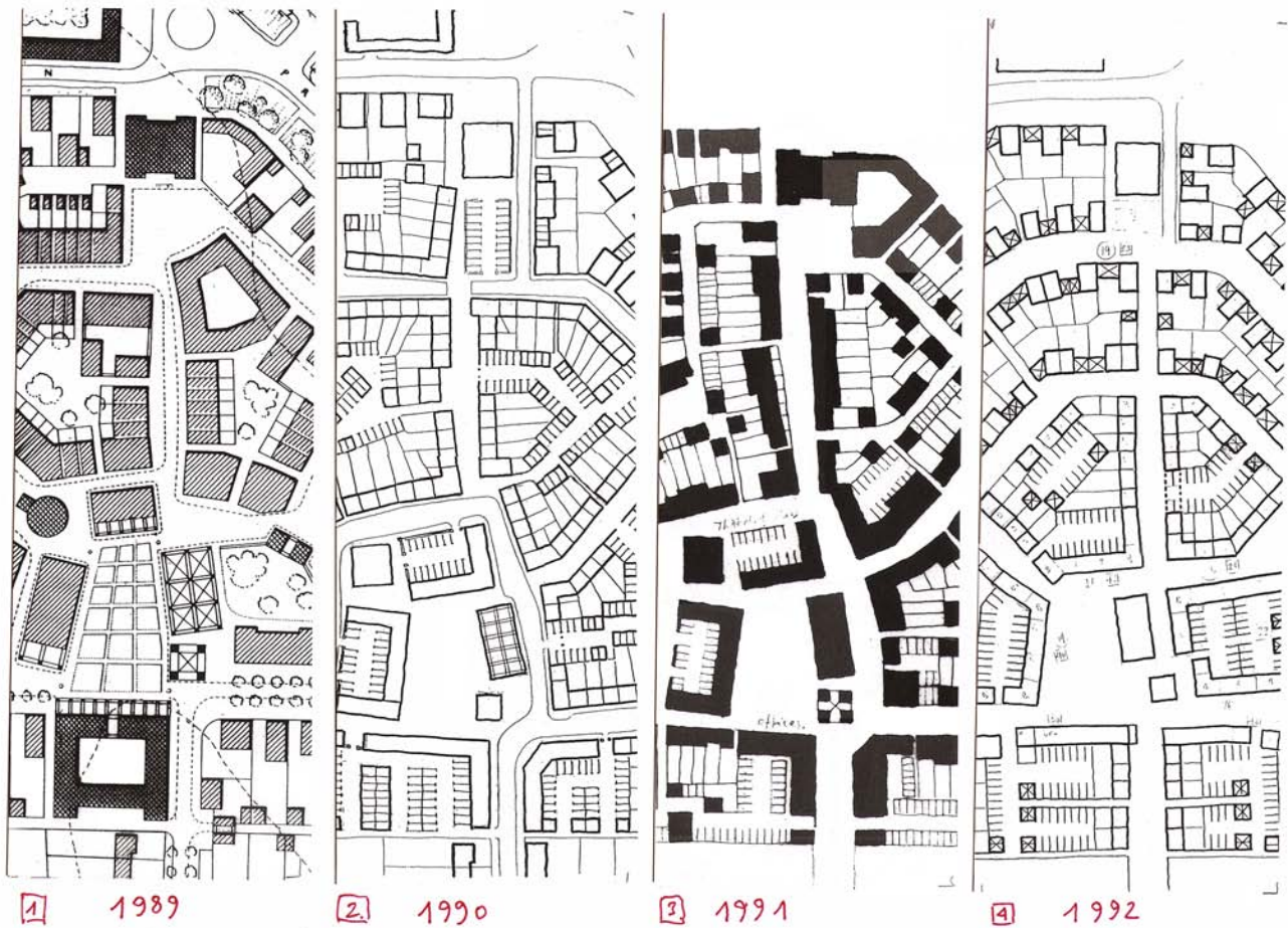
Figures 5.18 and 5.19: Longmoor Street, Poundbury, England. Plans. Léon Krier, 1989-1992. Successive plans trace the evolution of the Longmoor Street design. Images courtesy of Léon Krier
