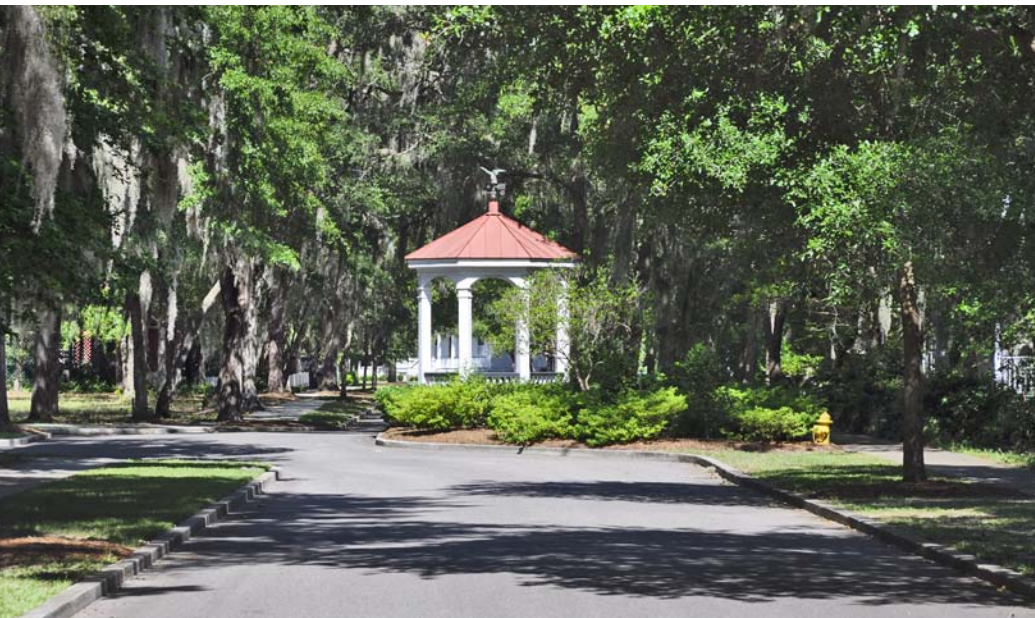
Figure 5.49: Newpoint Road, Lady's Island, South Carolina. V. Graham, R. Turner, and G. Cowart, 1991. Traffic calming as a byproduct of placemaking: drivers have to slow down to go around the gazebo that interrupts the straight street and terminates the vista.
