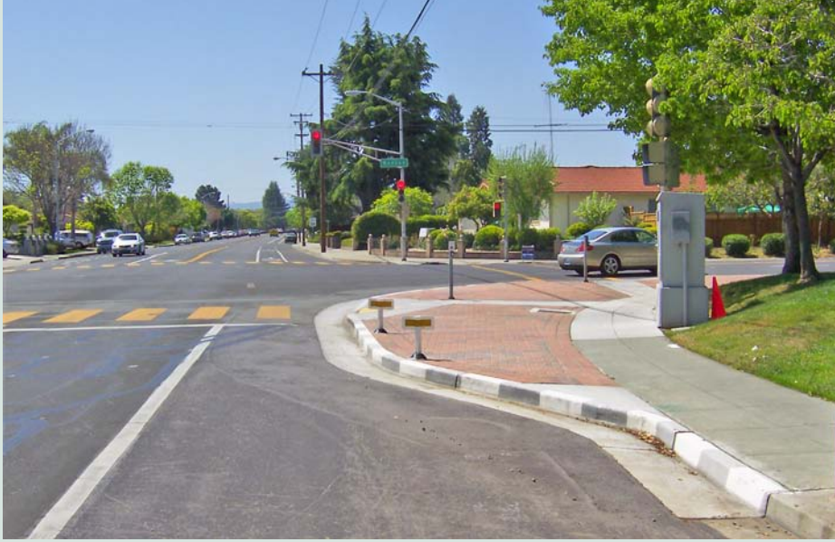
Figure 4.84: El Camino Real, Santa Clara, California. The road is wide, the buildings alongside the road do not enclose the space, and the scale of the auto-centric road is boring for the pedestrian. In this situation, the bumpout may make it psychologically easier for the occasional pedestrian to cross the street. But why would the pedestrian even be on the street here? This is not a detail that entices people out of their cars, and it is not a detail that would improve a walkable street. Image courtesy of the City of Los Altos
