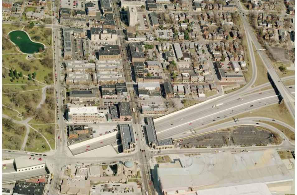
Figure 3.56: The Cap at Union Station, N High Street over I-670, Columbus, Ohio. Aerial view, looking north. Image courtesy of Pictometry International Corp. Copyright 2013
