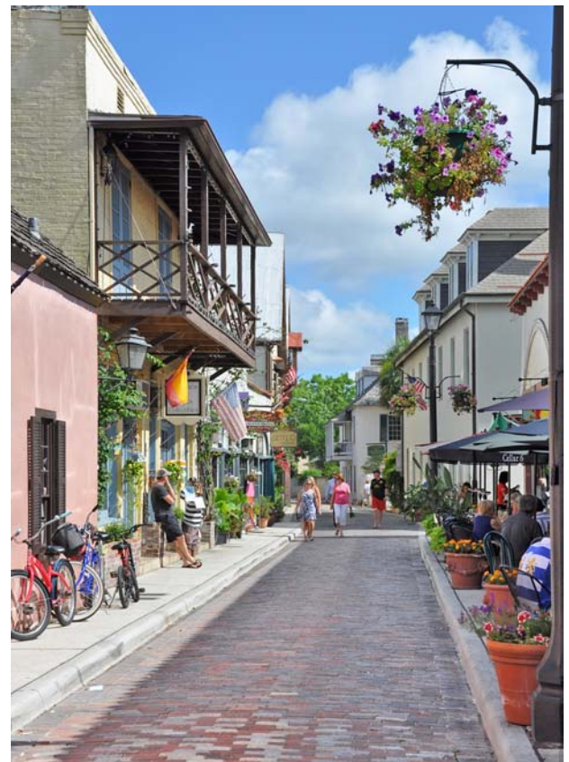
Figure 2.119: Aviles Street, St. Augustine, Florida. Small is beautiful: a single narrow lane, tightly spaced buildings, and the slight cant combine to make one of the most comfortable “shared space” streets in America.
