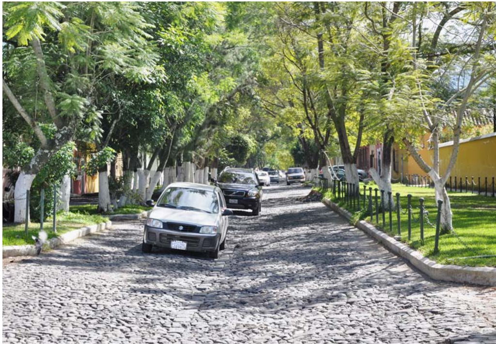
Figure 2.148: La Alameda de Santa Rosa, Antigua, Guatemala. A rare exception in the city's streets, its formal rows of trees grow in wide swales on both sides of the inverted-crown roadway; high garden walls with zaguanes line the sidewalks (seen at right).
