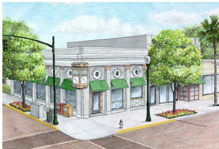
Figure 4.45: Park Avenue, Winter Park, Florida. Dover, Kohl & Partners, 1998. Design process sketch showing the restoration of simple intersection geometry, with no bulbouts. Small corner radii and elongated tree wells are also introduced. © 1998 Dover, Kohl & Partners
