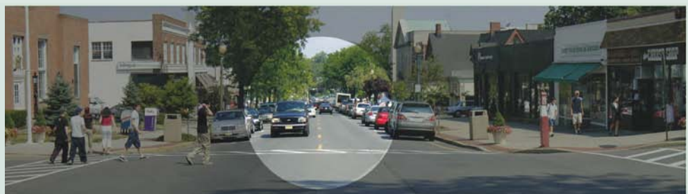
Figure 6.2: Cone of Vision Simulation. NACTO, 2010. The diminishing circles show how much small increases in speed decrease what a driver sees. The combination of reduced vision, the increased distances required for stopping, the greater amount of time needed for the driver to react to an obstacle, and the increased harm from impact as speeds go up show why speed kills. Image courtesy of NACTO
