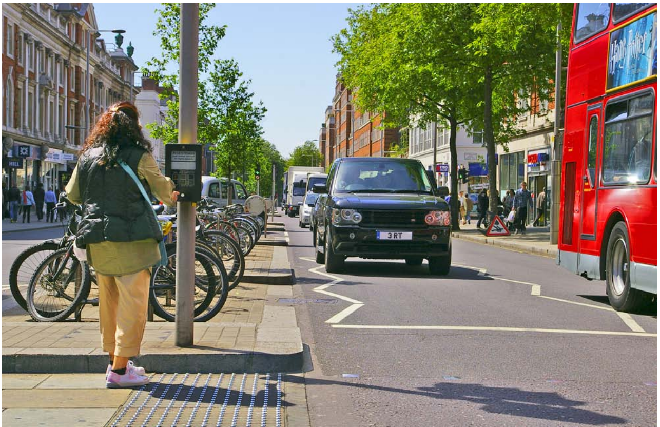
Figure 4.32: Kensington High Street, London, England. Royal Borough of Kensington and Chelsea, 2004. A limited palette of materials and colors gives the street simple elegance. Stainless steel studs replaced the usual yellow tactile blister paving at crosswalks.
