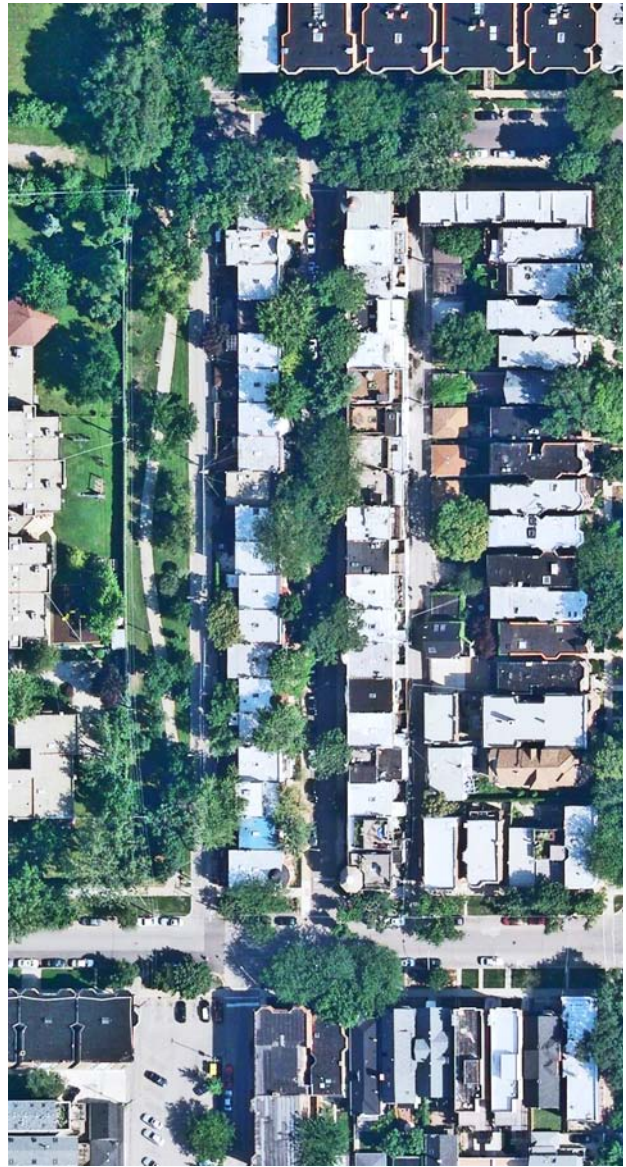
Figure 2.127: Alta Vista Terrace, Chicago, Illinois. J.C. Brompton, 1904. Satellite view. The shallow lots, compact building type, and narrow street (center) permitted the development of distinctive addresses despite the extremely tight parcel. Compare the shallow houses to the full-size rowhouses nearby (right and bottom). Image courtesy of Google Earth
