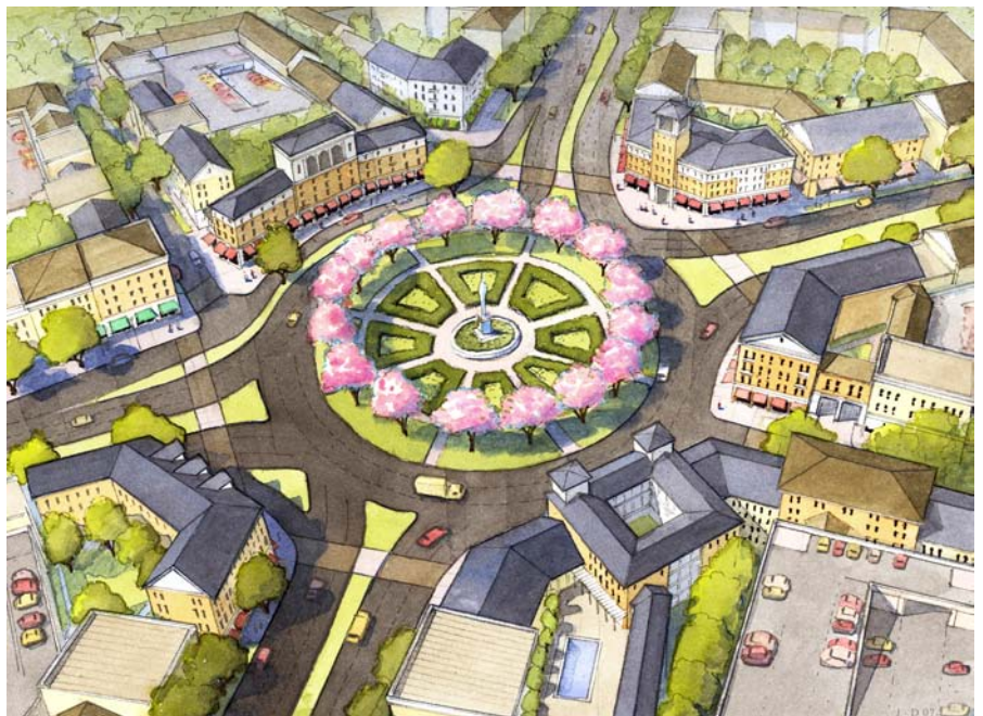
Figure 4.13: Fairfax Circle, Fairfax, Virginia. Dover, Kohl & Partners, 2008. Watercolor rendering, aerial view. The redesign includes correcting the traffic flow for slower speeds, planting a ring of trees within the circle to make its form more spatially evident, and amending development regulations to require space-shaping, street-oriented buildings. © 2008 Dover, Kohl & Partners
