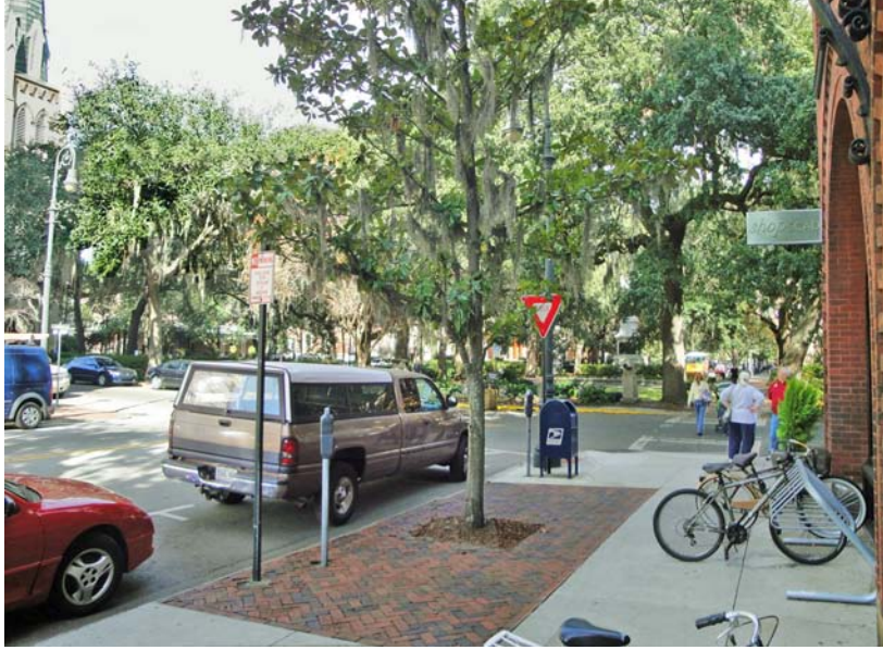
Figure 3.12: Bull Street at Madison Square, Savannah, Georgia. As the wide north-south streets come into the squares, they narrow to half the width and become part of the squares, functioning almost like shared spaces. The fact that they are not designed like roundabouts means that pedestrians feel comfortable crossing the street, while drivers have multiple distractions that force them to slow down to avoid hitting people and other cars. Image courtesy of Kevin Klinkenberg
