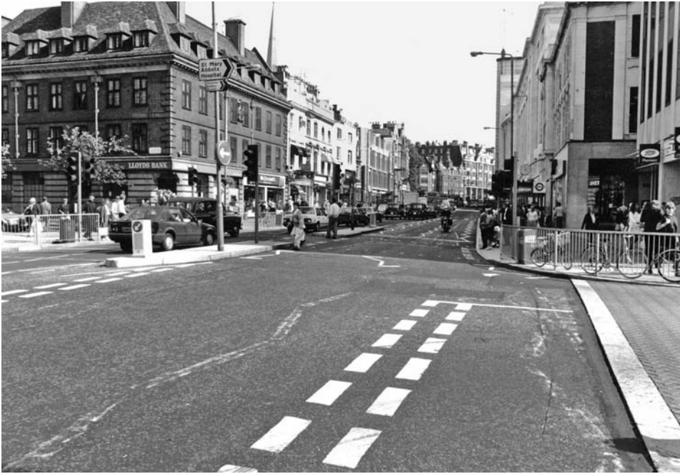
Figure 4.30: Kensington High Street, London, England. Before: Excessive, auto-scaled striping, signs, and railings took the joy out of the street experience. Property of the Royal Borough of Kensington and Chelsea
