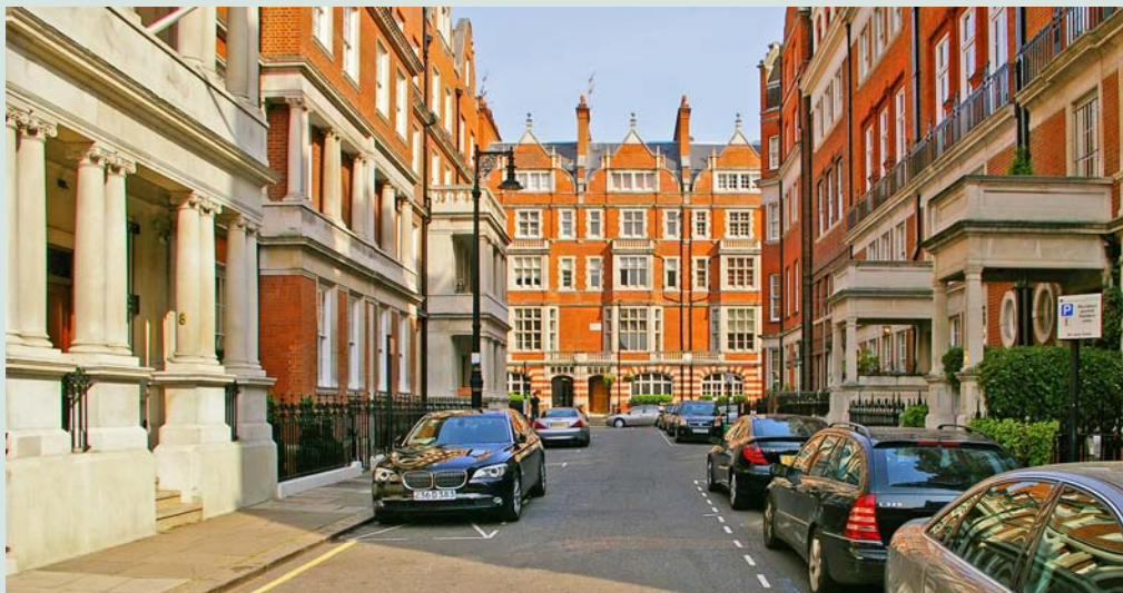
Figure 2.149: Balfour Place, London, England. View looking north toward Mount Street. The 'yield street' is a time-honored way to handle light two-way traffic without an unduly wide roadway.
