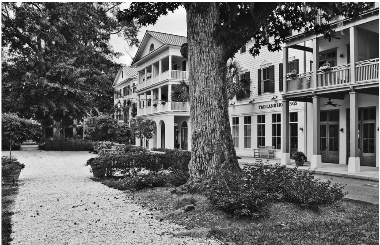
Figure 5.31: Le Chene Circle in Habersham, Beaufort, South Carolina. Duany Plater-Zyberk & Company, 1997. Looking southwest, showing pervious pea gravel path. The “Light Imprint” approach at Habersham does not call attention to itself as stormwater infrastructure, because it looks and feels like traditional Lowcountry placemaking.
