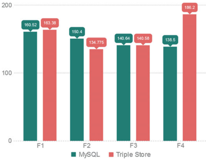
Fig. 9 Graphical representation of the average execution times of the four functions of the Ontology Service: comparison between the use of a MySQL database and a triple store
