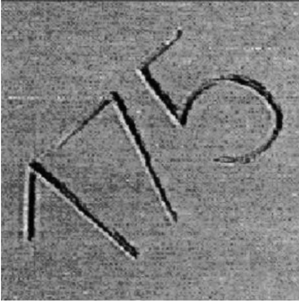
FIGURE F.8 Example of ATM usage: 9-nm lines in mica written with an AFM. (Courtesy: DFG-Center for Functional Nanostructures, Universität Karlsruhe, Germany).
