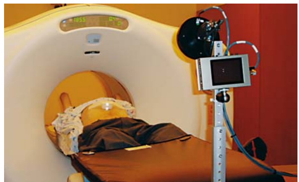
Fig. 45.4. 4D CT acquisition with an infrared camera tracking system consisting of an infrared source, CCD camera, and a reflecting block. The block is attached to the patient's abdomen, typically just inferior to the xiphoid process, and the motion of the block is captured by the camera
