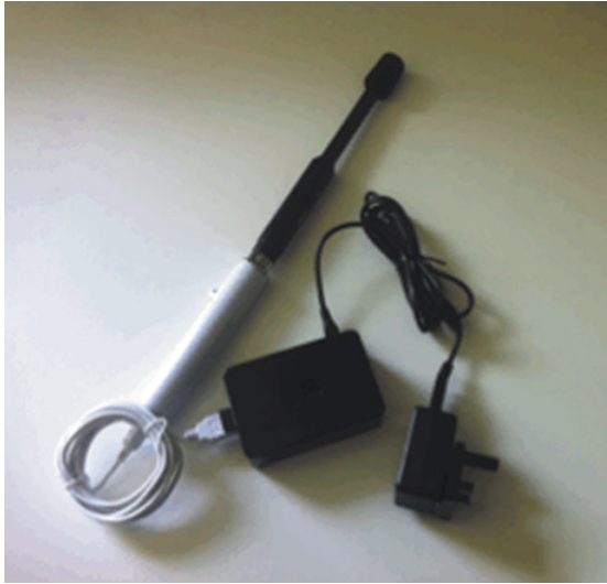
Fig. 18.1 Small computer with calibrated measurement microphone (Photograph by Christian Nold)
