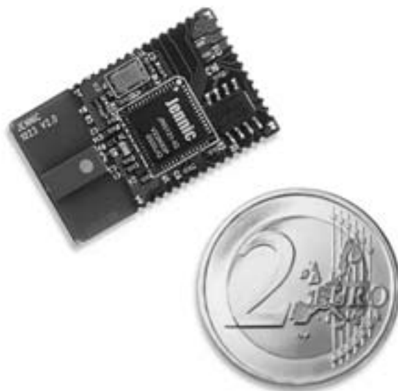
Figure 8. Coin-sized embedded controller module
