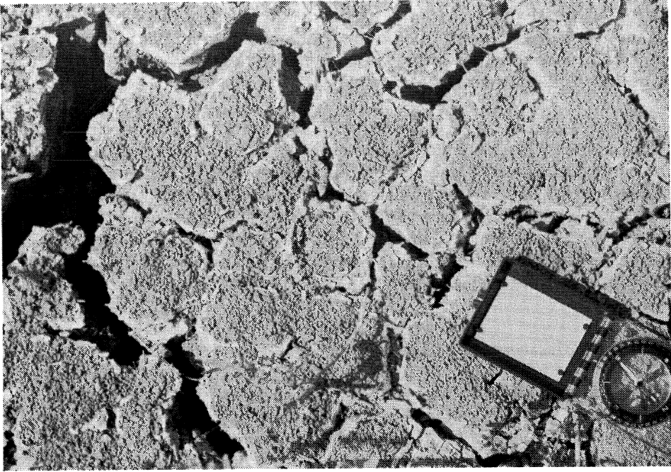
Figure 3: Sample LEW-2-1, a thin layer of very clayey, loose, sun-dried, angular chips. The chips lie on a relatively rigid layer of very light-grey-colored, sun-cracked, clayey silt.
