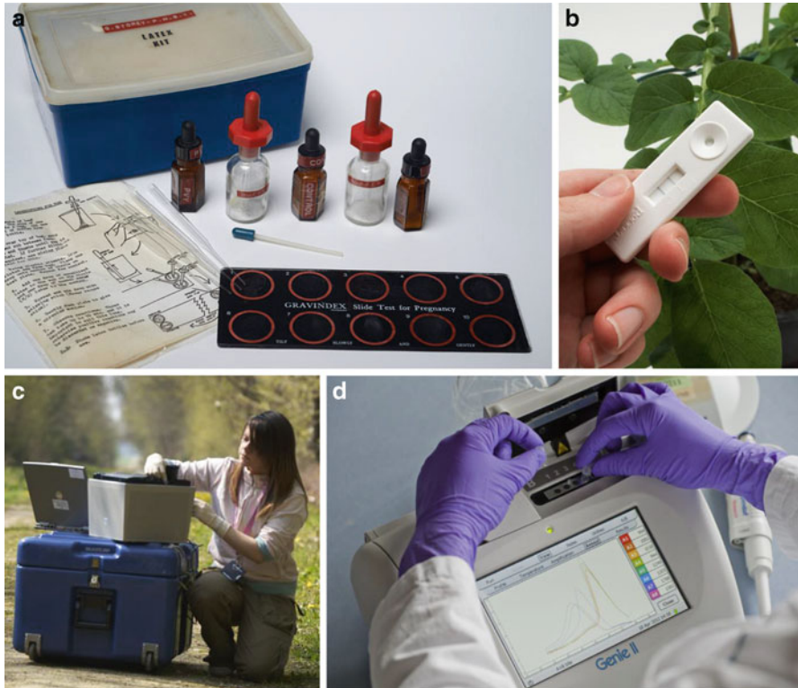
Fig. 1 Field test kits based on (a) Latex agglutination (b) Lateral flow devices (Forsite Diagnostics Ltd.) (c) Portable real-time PCR on the smart-cycler platform (Cepheid) and (d) LAMP on the Genie II platform (Optigene)
