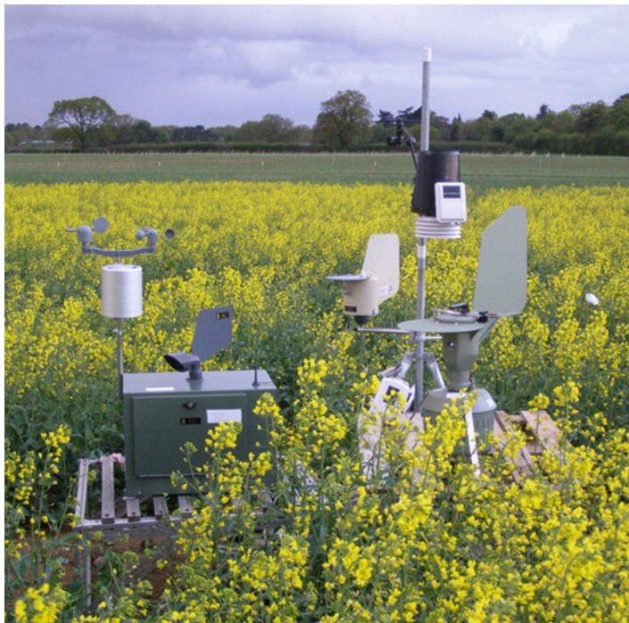
Fig. 4 SYield automated spore trap under validation with conventional air samplers at Rothamsted Research
