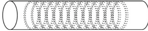
Fig. 9.5 Simplified axisymmetric stent model geometry showing cylindrical arterial segment and stent strut hoops (dashed)
