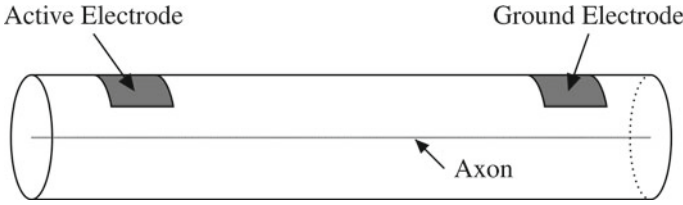
Fig. 6.15 Cylindrical nerve bundle with an internal axonal 1D edge (dashed line) stimulated by external cuff electrodes (shaded grey)
